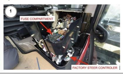
1) Begin by removing the passenger seat from the machine. This allows access to the steering controller compartment where the existing NAV controller is situated.
