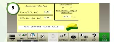
5) Ensure the receiver config settings are correct. Fore/Aft is the distance between the center of the fixed axle to the receiver. A TCM calibration will be required after changing these values. The maximum speed that the wheels can be turn can be set under 'Max Wheel Angle Velocity'. Default is 5°/sec.
