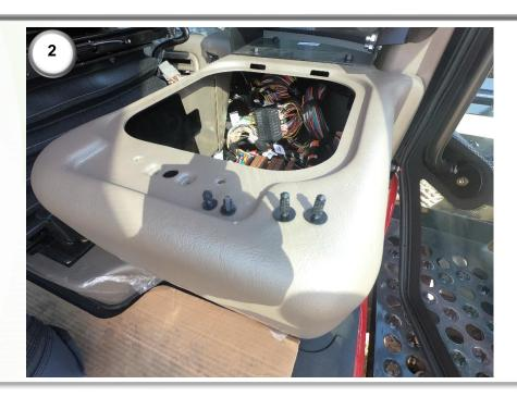
2) Locate the 40-way Deutsch connector. Plug the CNH Patriot interface harness (14) into this connector (an Allen key is also required to tighten it). Connect the Molex 46- way connector (11) into the ECU. Remove the Trimble NAV controller.
