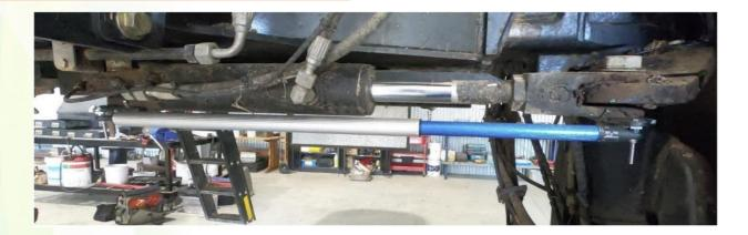
**5)** The linear potentiometer should be installed as shown. Disconnect the existing 'AUTOSENSE' sensor at the 4-way connector and connect the new sensor, ensuring to affix the harnessing in such as way that it cannot be damaged.
