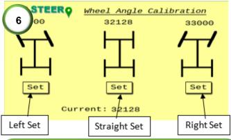
6) Calibrate the wheel angle sensor (WAS) limits. Ensure the current reading angle is not reading 0. Turn the steering wheel full lock left and press the left set button. Turn the wheel full lock right and press the right set button. Turn the wheel to dead straight and press the straight set button. Check the values above each set point to see if they've changed. Repeat the straight calibration using the WAS calibration procedure in step 10.
