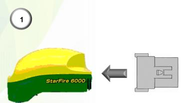
**1)** Install the SolSteer GS3 harness to provide the receiver and display with power and CAN. It can be easier to remove the 12-way connector for the receiver. Take note of the Pin outs.
