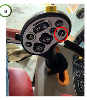
**8)** For the Case models engage the steering by pressing the auto engage button shown.
