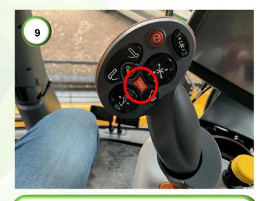
**9)** For the CNH models engage the steering by pressing the auto engage button shown.
