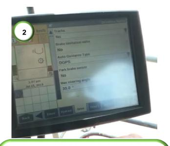
2) The machine type on the display will go to combine harvester and the recording source will go to 'AUTO'. This means the GreenStar is ready to record yield and moisture. Ensure the machine is ready to accept steering commands by selecting on the Intelliview screen: Toolbox > Drive > Auto guidance Type and set it to DGPS.
