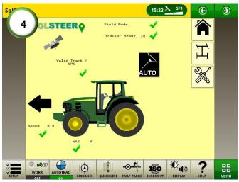
**4)** When there is a valid track selected, a valid GPS signal and the vehicle is ready to engage, all pre-acquisitions should be ticked.
