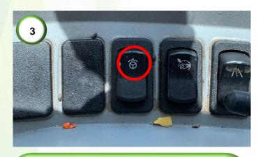
**3)** Every time the machine is started, the guidance must be armed on the combine. This is done by pressing the steering button on the side console on a 9.90 machine. If the machine is a 9090-type machine, the steering rocker switch must be held, and the steering wheel moved at the same time. The machine will then beep, and a steering wheel icon will appear on the CNH display.
