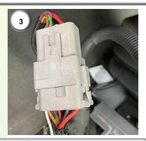
**3)** Locate the 12-way Deutsch connectors attached to the seat. Plug the two 12-way connectors (7 and 8) into these two connectors. The power for the GreenStar equipment is taken from this connector. If the CNH combine is an older series (CR 2007-2013 series) locate a switch power source and attach the CNH interface harness to the switch power source using a 12-way Deutsch connector.
