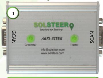
1) Turn the ignition on and wait for the GreenStar to turn on. Note that the LED's on the Agri-Steer module will be red until communication is made with the GreenStar display. The GreenStar will then display the 'Automatic Guidance System' warning and the LED's will flash green.
