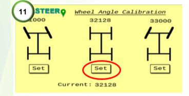
**11)** While tracking on-line, press the straight set button in the setup page. This will then save the dead center point of the wheel angle sensor (WAS).
