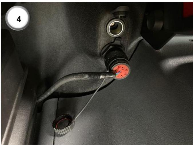
**4)** Locate the diagnostic port next to the passenger seat and connect the harness plug labelled 'DIAG'. NOTE: This socket may be in the fuse cupboard next to the key.
