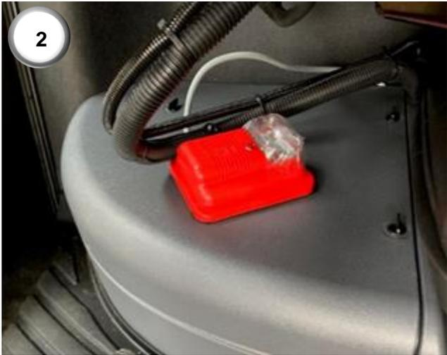
**2)** Locate and remove the cover next to the driver's seat. This is where the module can be stored.
