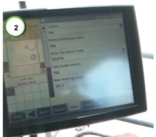
**1)** Turn the ignition on and wait for the GreenStar to turn on. Note that the LED's on the Agri-Steer module will be red until communication is made with the GreenStar display. The GreenStar will then display the 'Automatic Guidance System' warning and the LED's will flash green.
