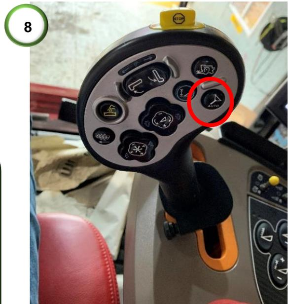
8) For the Case models engage the steering by pressing the auto engage button shown.
