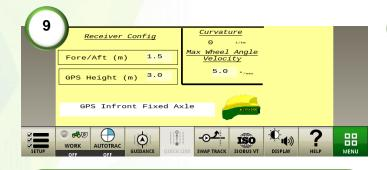
**9)** Ensure the receiver config settings are correct. Fore/Aft is the distance between the center of the fixed axle to the receiver. A TCM calibration will be required after changing these values. The maximum speed that the wheels can be turn can be set under 'Max Wheel Angle Velocity'. Default is 5°/sec.
