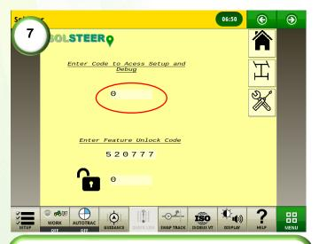
**7)** Access the setup and dealer lever diagnostics page. Enter the code 835 into the debug field.
