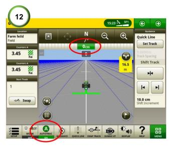
**12)** Engage the steering and drive at about 4kph. Wait for the cross-track error to be holding a stable value around 0cm.
