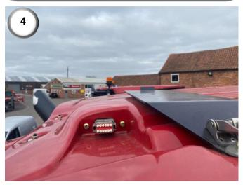
**4)** Locate the 12-way Deutsch connecter on the roof. Remove the plug that is located in the socket and insert the 12-way connector plug of the roof adaptor (2). Insert the 12-way connector socket of the roof adaptor into the StarFire receiver.
