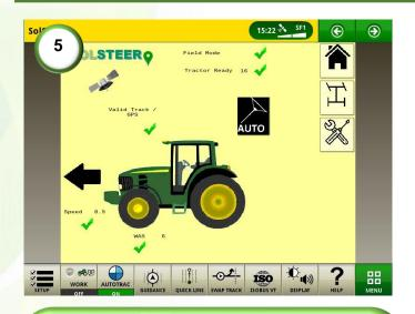
**5)** When there is a valid track selected, a valid GPS signal and the vehicle is ready to engage, all pre-acquisitions should be ticked.
