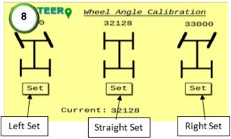
**8)** Calibrate the wheel angle sensor (WAS) limits. Ensure the current reading angle is not reading 0. Turn the steering wheel full lock left and press the left set button. Turn the wheel full lock right and press the right set button. Turn the wheel to dead straight and press the straight set button. Check the values above each set point to see if they've changed. Repeat the straight calibration using the WAS calibration procedure in step 6 next page.
