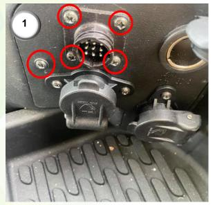
1) Locate the 9-way ISOBUS socket at the back-right corner of the cab. Remove the screws that hold the panel in place. Also remove the screws that hold the 9-way ISOBUS panel mount socket to the panel. Connect the permanent power wire (4) to the permanent power source (this is located in the connector underneath the 9-way connector).
