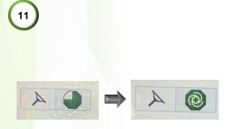
11) In the Case display, ensure that the steering icon has changed from <sup>3</sup>/<sub>4</sub> pie to a full pit chart as it does on the John Deere GreenStar display.
