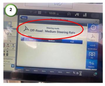
**2)** Ensure that the steering mode is in 'Off-Road' mode. This must be activated for external guidance systems to work. If the steering mode instead shows 'On-Road' mode then see the next step.
