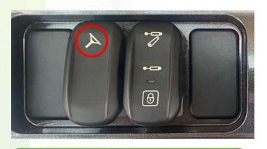
**3)** If the system instead shows 'On-Road' mode then press the roading switch in the headliner. This will put the steering mode back into 'Off-Road' mode.
