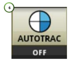
6) Once an A-B line is set, arm the GreenStar for steering. This is done by pressing the 'AUTOTRAC' button at the bottom of the screen. Once three-quarters of the circle are filled the system is ready to engage.
