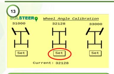
**13)** While tracking on-line, press the straight set button in the setup page. This will then save the dead center point of the wheel angle sensor (WAS).
