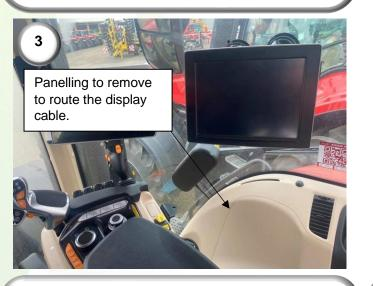
**3)** Feed the display cable underneath the paneling on the right-hand side of the cab, removing any paneling where necessary. Plug the 26-way display cable (3) into the John Deere display.
