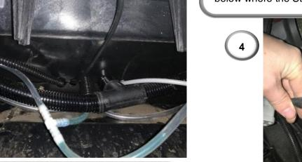
4) Check if the machine has the 'OSI Ready' harness installed. This is a 6-way Deutsch connector (usually located under the panel behind the seat) with 5 wires into it. If the OSI harness is there, connect the Lexion adaptor (CL/006) here with the male 6-way Deutsch connector (8).
