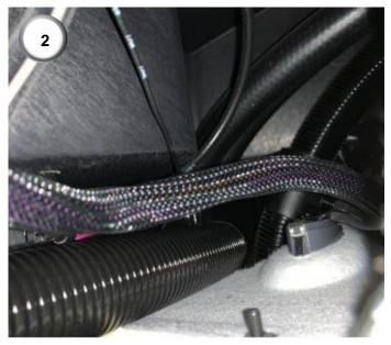
2) Locate the large diameter conduit. This runs from the back right-hand corner of the cab within the roof liner to the front center section outside the cab (between the top of the windscreen and below where the StarFire receiver would sit)
