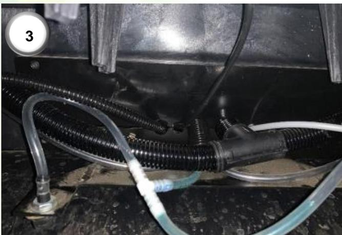
**3)** Remove the necessary panels and lights to gain access behind the 'Lexion' panel (between the top of the windscreen and below where the StarFire receiver would sit) section at the front of the cab. This reveals the outer end of the conduit. Remove the 12-way connector (2) of the GS4 harness. Thread the harness from the cab, through the conduit, and to the outside of the cab. Reinstall the 12-way connector. Pinouts are found on page 13.
