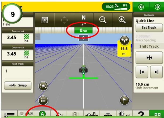
**9)** Engage the steering and drive at about 4kph. Wait for the cross-track error to be holding a stable value around 0cm.
