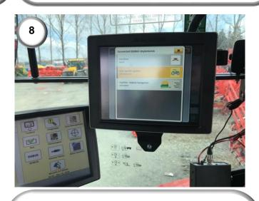
8) Run the 12-way connector of the GS3 harness to the roof (2) and plug in the display using the 26-way connector plug (4). AFTER the GS3 is installed, connect the 12-way connectors of the GS3 harness and the CNH Magnum interface harnesses together (5 & 7). IMPORTANT! Do not connect the GS3 harness to the CNH Magnum interface harness until the CNH Magnum interface harness has been fitted. This could result in a short circuit occurring!
