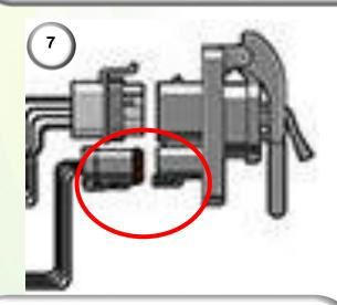
7) If the tractor is ISOBUS, remove the 4-way Deutsch connector on the back of the ISOBUS plug on the back of the tractor. Plug the 4-way male Deutsch connector of the CNH Magnum interface harness (13) in here. This will provide the system with ISOBUS implement communication.
