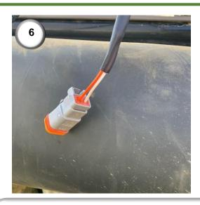
6) Disconnect the two-way Deutsch labelled 'enable' or 'activate' from the solenoid. Plug in the male two- way Deutsch connector from the CNH Magnum valve extension cable (14). Connect the other end of the CNH Magnum valve extension cable (15) to the CNH Magnum interface harness.
