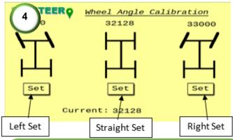
4) Calibrate the wheel angle sensor (WAS) limits. Ensure the current reading angle is not reading 0. Turn the steering wheel full lock left and press the left set button. Turn the wheel full lock right and press the right set button. Turn the wheel to dead straight and press the straight set button. Check the values above each set point to see if they've changed. Repeat the straight calibration using the WAS calibration procedure in step 6 next page.
