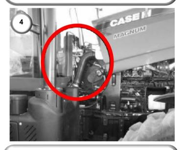
**4)** For this install, a cable must be connected to the 'enable' solenoid on the steering valve. This activates the auto-steer hydraulics.
