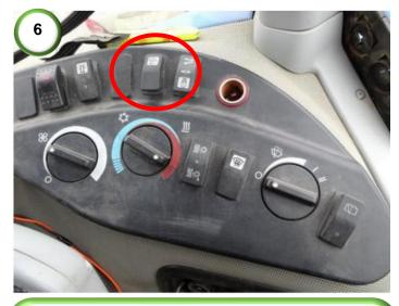
**6)** To steer, ensure the 'AUTO' rocker switch on the right-hand pillar is switched up. **IMPORTANT!** Ensure this switch is in the OFF position during road travel to prevent accidental engagement.
