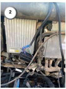
2) Locate the 40-way Deutsch connector. Plug the CNH Magnum interface harness (6) into this connector (an Allen key is also required to tighten it). Connect the Molex 46- way connector (9) into the ECU. Remove the Trimble Nav controller, and bolt the Agri-Steer ECU to the remaining bolt stubs.
