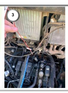
**3)** Locate a permanent power source (+12V) for the system. Join the red wire from the CNH Magnum interface harness to the permanent 12V+ supply. This will provide power to the display and receiver.
