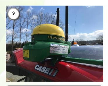
9) Mount the Starfire receiver on the roof as far forward and as central as possible. Plug the 12-way connector of the GS3 harness into the Starfire receiver (2). Note: the Starfire roof bracket is not included. Installation is now complete.
