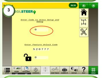
**3)** Access the setup and dealer lever diagnostics page. Enter the code 835 into the debug field.
