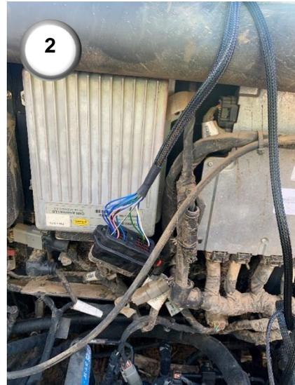
**1)** Locate where the NAV controller would normally be fitted (on a Case this is behind the cab on the outside). On a New Holland it is behind the passenger seat in the cab. Remove the cover to expose the NAV connections.
