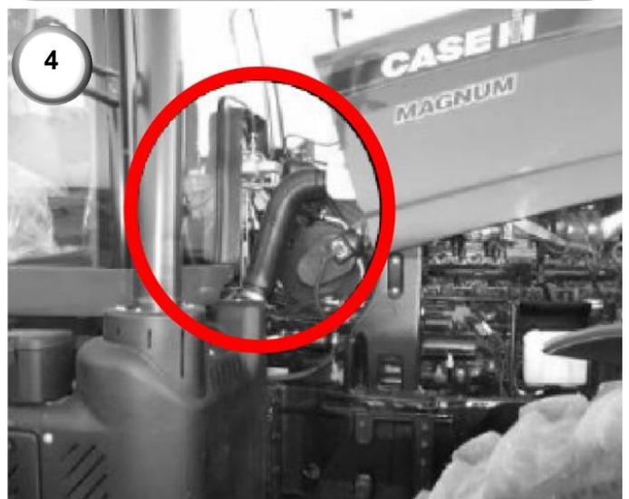
**3)** Locate a permanent power source (+12V) for the system. Join the red wire from the CNH Magnum interface harness to the permanent 12V+ supply. This will provide power to the display and receiver.
