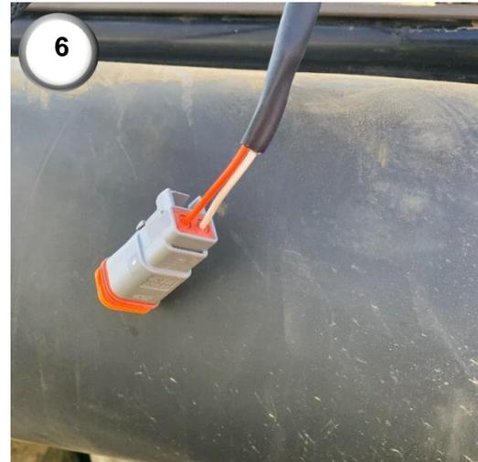
**6)** Disconnect the two-way Deutsch labelled 'enable' or 'activate' from the solenoid. Plug in the male two- way Deutsch connector from the CNH Magnum valve extension cable (14). Connect the other end of the CNH Magnum valve extension cable (15) to the CNH Magnum interface harness.
