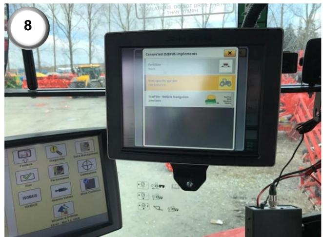
**8)** Run the 12-way connector of the GS3 harness to the roof (2) and plug in the display using the 26-way connector plug (4). **AFTER** the GS3 is installed, connect the 12-way connectors of the GS3 harness and the CNH Magnum interface harnesses together (5 & 7). **IMPORTANT!** Do not connect the GS3 harness to the CNH Magnum interface harness until the CNH Magnum interface harness has been fitted. This could result in a short circuit occurring!
