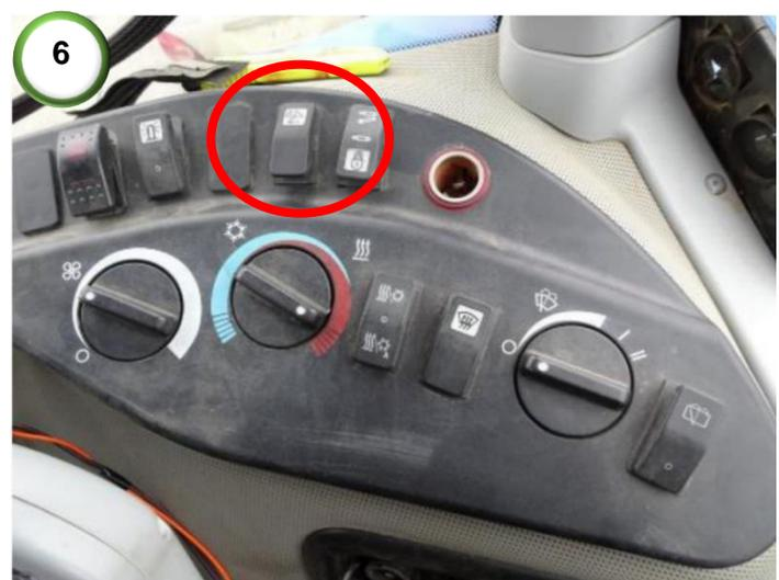
6) To steer, ensure the 'AUTO' rocker switch on the right-hand pillar is switched up. **IMPORTANT!** Ensure this switch is in the OFF position during road travel to prevent accidental engagement.
