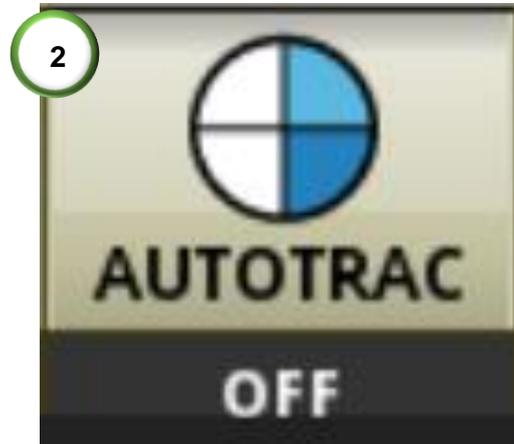
2) Once an A-B line is set, arm the GreenStar for steering. This is done by pressing the 'AUTOTRAC' button at the bottom of the screen. Once three-quarters of the circle are filled the system is ready to engage. **IMPORTANT!** Disarm the GreenStar steering with two-quarters of the circle full when travelling on public roads.
