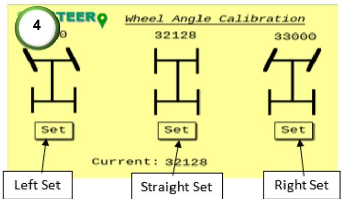
4) Calibrate the wheel angle sensor (WAS) limits. Ensure the current reading angle is not reading 0. Turn the steering wheel full lock left and press the left set button. Turn the wheel full lock right and press the right set button. Turn the wheel to dead straight and press the straight set button. Check the values above each set point to see if they've changed. Repeat the straight calibration using the WAS calibration procedure in step 6 next page.
