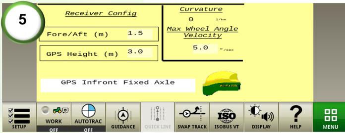
5) Ensure the receiver config settings are correct. Fore/Aft is the distance between the center of the fixed axle to the receiver. A TCM calibration will be required after changing these values. The maximum speed that the wheels can be turn can be set under 'Max Wheel Angle Velocity'. Default is 5°/sec.
