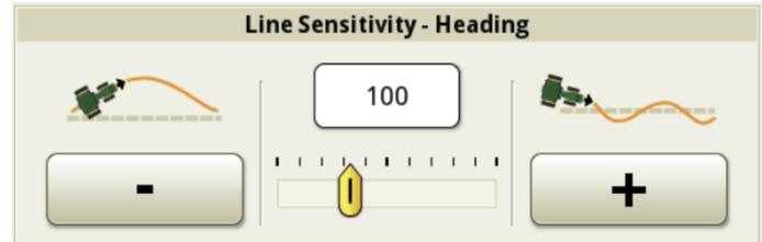
**6)** Adjust this parameter if the heading error is oscillating, the higher the number, the more sensitive to heading error the system will become.
