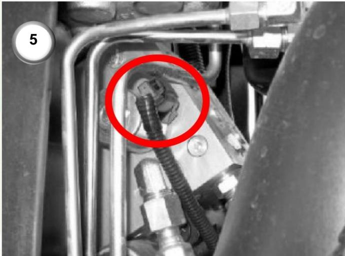
**5)** Run the cable of the CNH Magnum valve extension cable under the cab and to the steering valve as shown in the picture.
