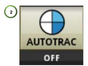
2) Once an A-B line is set, arm the GreenStar for steering. This is done by pressing the 'AUTOTRAC' button at the bottom of the screen. Once three-quarters of the circle are filled the system is ready to engage.
