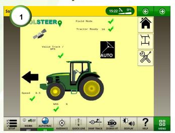
1) When there is a valid track is selected, a valid GPS signal and the vehicle is ready to engage, all pre-acquisitions should be ticked.
