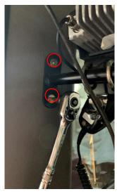
1) Ensure that the machine has the wheel angle sensor (WAS) as shown in the picture. If it does not, the machine requires the analogue steering system. Contact SolSteer for more information.
