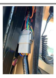
**3)** Locate the 12-way DTM connector behind the cover.
