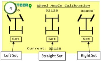
4) Calibrate the wheel angle sensor (WAS) limits. Ensure the current reading angle is not reading 0. Turn the steering wheel full lock left and press the left set button. Turn the wheel full lock right and press the right set button. Turn the wheel to dead straight and press the straight set button. Check the values above each set point to see if they've changed. Repeat the straight calibration using the WAS calibration procedure in step 6 on next page.
