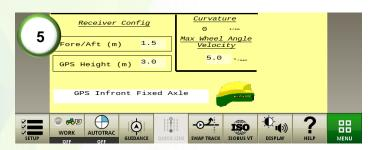
**5)** Ensure the receiver config settings are correct. Fore/Aft is the distance between the center of the fixed axle to the receiver. A TCM calibration will be required after changing these values. The maximum speed that the wheels can be turn can be set under 'Max Wheel Angle Velocity'. Default is 5°/sec.
