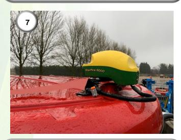
7) Connect the CNH roof harness into the roof of the machine using the 12-way connector plug (6) and plug the adaptor into the StarFire using the connector socket (7).
