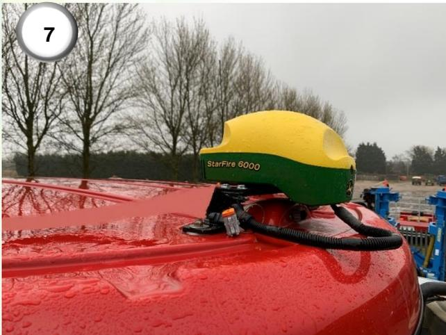
**7)** Connect the CNH roof harness into the roof of the machine using the 12-way connector plug (6) and plug the adaptor into the StarFire using the connector socket (7).
