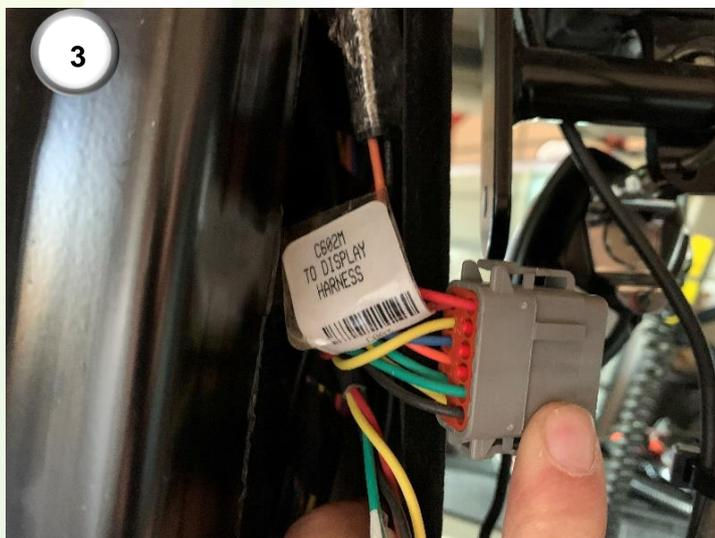
**3)** Locate the 12-way DTM connector behind the cover.
