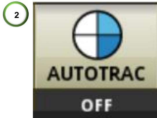
2) Once an A-B line is set, arm the GreenStar for steering. This is done by pressing the 'AUTOTRAC' button at the bottom of the screen. Once three-quarters of the circle are filled the system is ready to engage. **IMPORTANT!** Disarm the GreenStar steering with two-quarters of the circle full when travelling on public roads.
