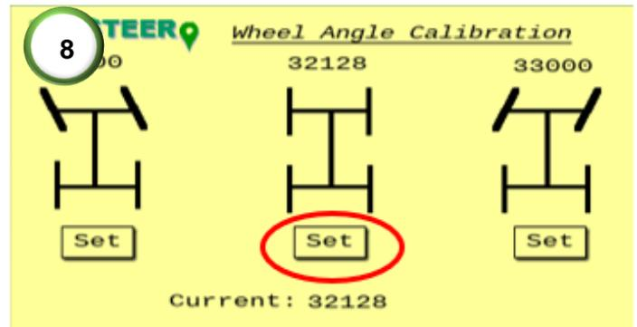
**8)** While tracking on-line, press the straight set button in the setup page. This will then save the dead center point of the wheel angle sensor (WAS).
