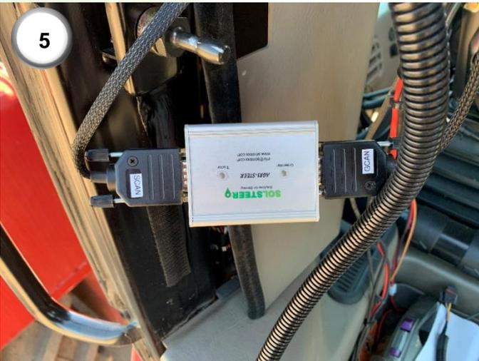
**5)** Connect the Agri-Steer module. The GCAN D-Sub connector (5) connects to the Greenstar side and the SCAN D-Sub connector (4) connects to the tractor side.
