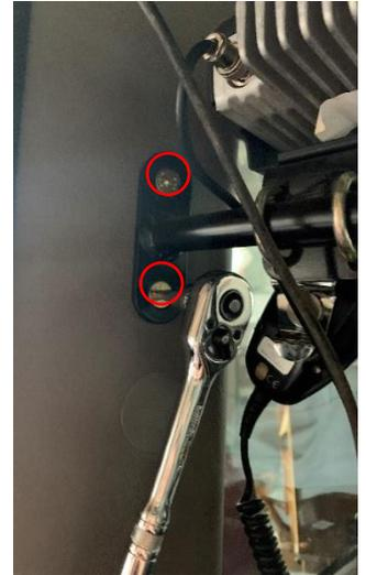
**2)** Remove the right-hand door stop. It might also be necessary to remove the mounting bar bolts as shown.
