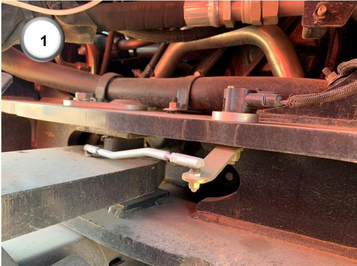
**1)** Ensure that the machine has the wheel angle sensor (WAS) as shown in the picture. If it does not, the machine requires the analogue steering system. Contact SolSteer for more information.
