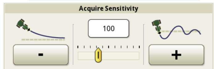
4) Adjust this parameter until the acquisition is satisfactory. The higher this number, the more aggressive the vehicle will turn onto the line.
