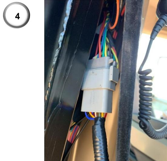
**4)** Connect the CNH Agri-Steer Cab Harness using one or both 12-way DTM connectors (1 and 2), depending on whether there are two connectors already connected.
