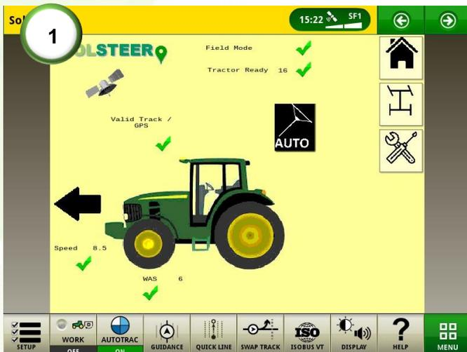
1) When there is a valid track is selected, a valid GPS signal and the vehicle is ready to engage, all pre-acquisitions should be ticked.
