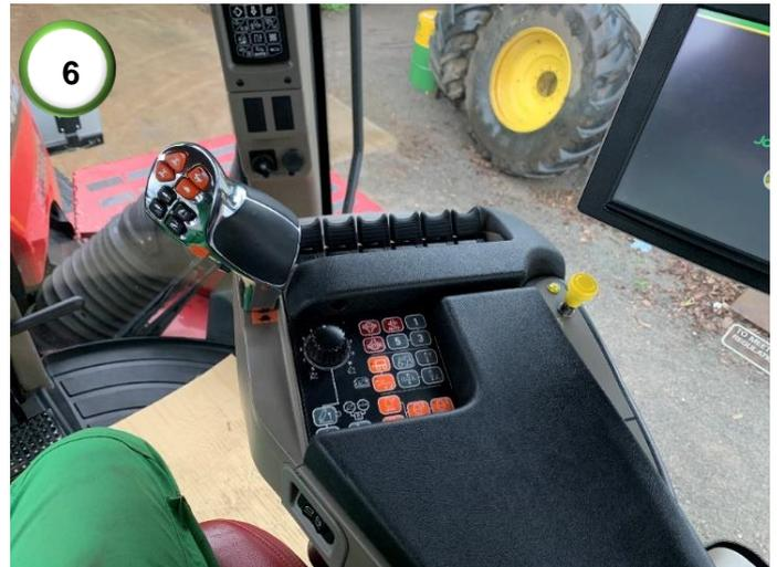
**6)** Use the HMS button on the joystick or the engage button on the pad to engage the steering.
