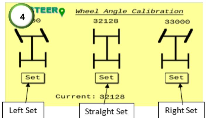
4) Calibrate the wheel angle sensor (WAS) limits. Ensure the current reading angle is not reading 0. Turn the steering wheel full lock left and press the left set button. Turn the wheel full lock right and press the right set button. Turn the wheel to dead straight and press the straight set button. Check the values above each set point to see if they've changed. Repeat the straight calibration using the WAS calibration procedure in step 6 on next page.
