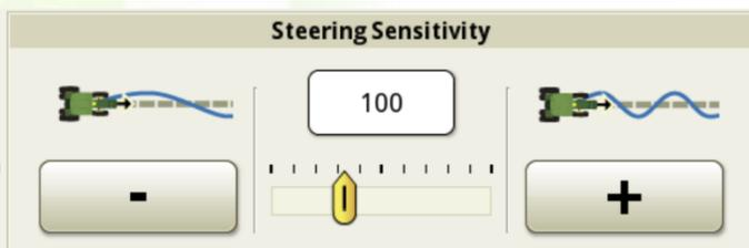
3) Adjust this parameter to make the system more aggressive. The higher this number, the more the wheels will turn for the same amount of error.
