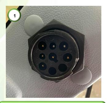
**1)** Locate the 9 way in-cab socket located on the back-right upright pillar of the cab.
