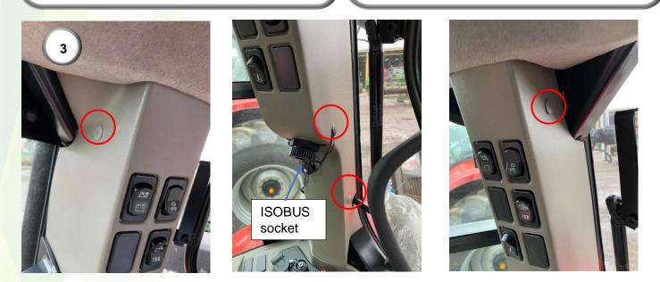
**3)** Locate the 9-way ISOBUS socket at the back-left column of the cab. Remove the panel where the ISOBUS socket is located, by removing the plastic caps shown and unscrewing the screws beneath them. Replace the 9 way in-cab ISOBUS socket with the same socket of the CNH Agri-Steer harness (10). Connect the remaining 9 way ISOBUS socket of the CNH Agri-steer harness (8) to the 9 way ISOBUS socket that had just been removed.
