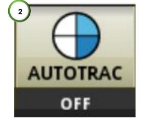
1) Turn the ignition on and wait for the GreenStar to turn on. Note that the LED's on the Agri-Steer module will be red until communication is made with the GreenStar display. The LED's will then flash orange until there is communication with the GreenStar display. 2) Once an A-B line is set, arm the GreenStar for steering. This is done by pressing the 'AUTOTRAC' button at the bottom of the screen. Once three-quarters of the circle are filled the system is ready to engage.
