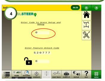
**4)** Access the setup and dealer lever diagnostics page. Enter the code 835 into the debug field.
