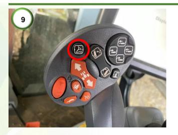
**9)** Engage the steering by pressing the 'auto' button on the joystick.
