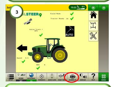
**3)** Locate the Solsteer page by clicking on the ISOBUS VT icon. When there is a valid track selected, a valid GPS signal and the vehicle is ready to engage, all pre-acquisitions should be ticked.
