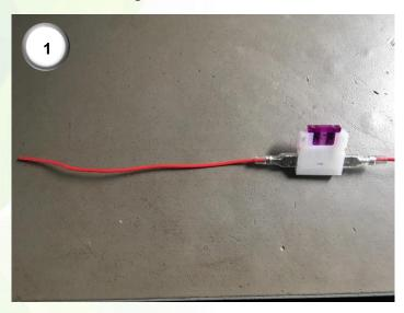
**1)** Connect the CNH Agri-steer interface harness to a permanent power source with the red wire.
