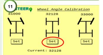
**11)** While tracking on-line, press the straight set button in the setup page. This will then save the dead center point of the wheel angle sensor (WAS).
