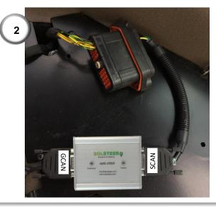
**2)** Remove the NAV controller panel to the left of the driver's seat and locate the 40-way Deutsch connector. Plug the Agri-steer loom labelled 'SCAN' here and connect the other end to the port labelled 'GCAN' on the CNH Agristeer harness (14).
