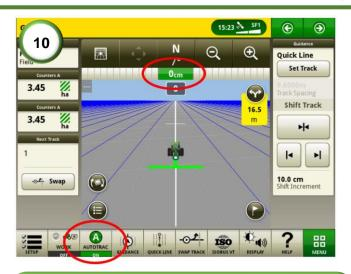
**10)** Engage the steering and drive at about 4kph. Wait for the cross-track error to be holding a stable value around 0cm.
