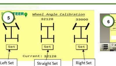
**5)** Calibrate the wheel angle sensor (WAS) limits. Ensure the current reading angle is not reading 0. Turn the steering wheel full lock left and press the left set button. Turn the wheel full lock right and press the right set button. Turn the wheel to dead straight and press the straight set button. Check the values above each set point to see if they've changed. Repeat the straight calibration using the WAS calibration procedure in step 8.
