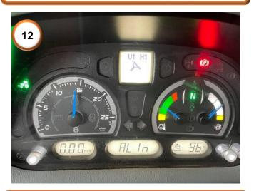
**12)** When 'AI In' shows the system is ready to start the auto-calibration routine. Press 'auto'.
