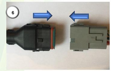
**6)** Connect the 12-way connector of the CNH Agri-steer harness (7) to the 12 way connector of the GS3 harness (6).
