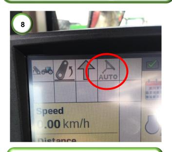
**8)** A steering wheel with 'auto' will then be displayed on the tractors display. The system is now ready to engage.
