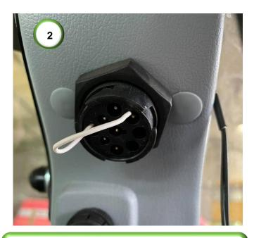
**2)** Use a wire connect pins 'B' and 'G'. Turn the tractor on.
