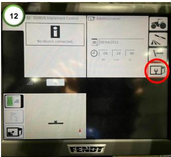
**11)** For the system to work, ISOBUS must be turned on in the Fendt UT. To do this press the spanner icon.
