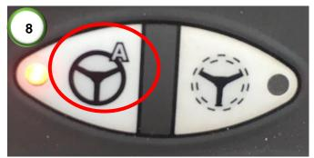
**8)** To engage, press the white steering engage button as shown. This can also be programmed to any button on the joystick via the Fendt terminal. **Note:** Moving the steering wheel at any time will disengage.
