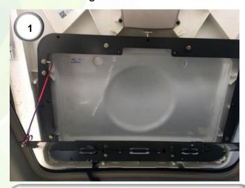
1) Locate and remove the inside roof panel where a standard receiver would be located. Mount the Agri-Steer here.
