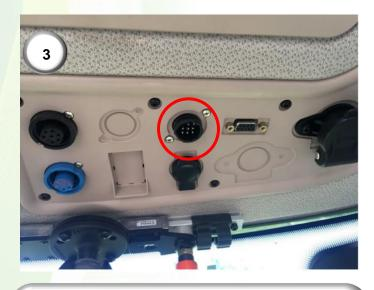
**3)** Locate the roof panel at the back of the cab and remove the bolts holding it in place. Remove the plastic panel covering the right/back cab upright.
