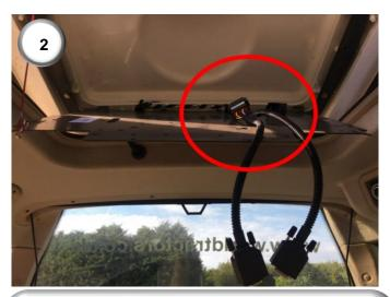
2) Locate the 12-way Connector in the cab and connect it to the 12-way Connector socket (9). Plug both D-Sub Connectors (10 and 12) into the Agri-Steer Module (11) with GCAN in the GCAN side and the SCAN in the SCAN side.
