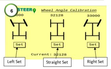
6) Calibrate the wheel angle sensor (WAS) limits. Ensure the current reading angle is not reading 0. Turn the steering wheel full lock left and press the left set button. Turn the wheel full lock right and press the right set button. Turn the wheel to dead straight and press the straight set button. Check the values above each set point to see if they've changed. Repeat the straight calibration using the WAS calibration procedure in step 9 on next page.
