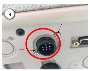
**4)** Remove the two screws holding the female 9-pin ISO socket. Replace the ISO socket with the identical ISO socket on the GCAN adaptor harness (7).
