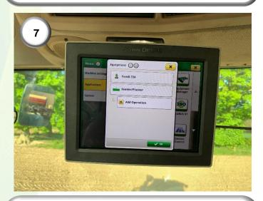
7) Mount the Greenstar Display (3) and connect the 26-way Connector plug (4) of the GS3 loom to the Greenstar Display in the 'Main' or 'Machine' socket.
