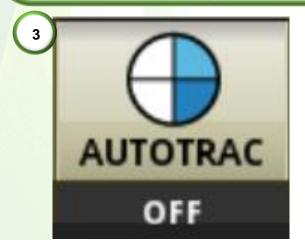
3) Once an A-B line is set, arm the GreenStar for steering. This is done by pressing the 'AUTOTRAC' button at the bottom of the screen. Once three-quarters of the circle are filled the system is ready to engage.
