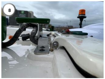
8) Mount the StarFire receiver on the roof as far forward and as central as possible. Run the StarFire cable with the 12- Way Connector Socket (2) along the roof and tighten it securely to the tractor. Join the Connector to the StarFire receiver.
