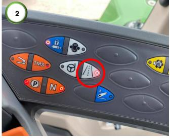
1) Turn the ignition on and wait for the GreenStar to turn on. Note that the LED's on the Agri-Steer module will be red until communication is made with the GreenStar display. The GreenStar will display 'Automatic Guidance System' warning and the LED's will start flashing green when the system is ready to use. **2)** To arm the Fendt Vario MT Vario MT 900 ready for steering press the right white button, to deactivate road mode. When unactive, the red LED will disappear.
