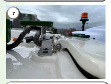
7) Mount the StarFire receiver on the roof as far forward and as central as possible. Run the StarFire cable with the 12- Way Connector Socket (2) along the roof and tighten it securely to the tractor. Join the Connector to the StarFire receiver.
