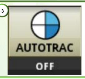
3) Once an A-B line is set, arm the GreenStar for steering. This is done by pressing the 'AUTOTRAC' button at the bottom of the screen. Once three-quarters of the circle are filled the system is ready to engage.
