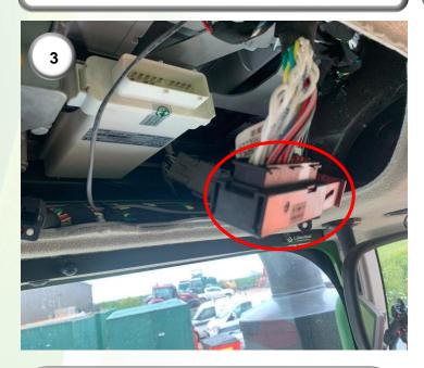
**3)** Disconnect the 29-way connector from the VD03 controller, by pulling open the tab on the side of the connector.
