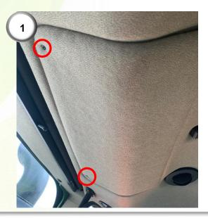
**1)** Locate and remove the inside roof panel by removing the two screws shown.
