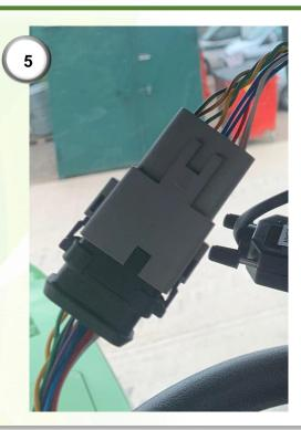
**5)** Connect the 12-way Deutsch connector plug of the GS3 harness (5) to the 12-way Deutsch connector socket of the Fendt Vario MT adaptor harness (6). Run the GS3 harness to the roof ready to connect to the StarFire receiver.
