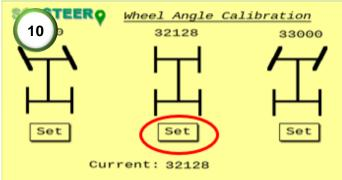
**10)** While tracking on-line, press the straight set button in the setup page. This will save the dead center point of the wheel angle sensor (WAS).
