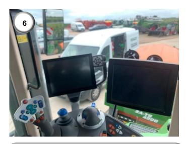
**6)** Mount the Greenstar Display (3) and connect the 26-way Connector plug (4) of the GS3 loom to the Greenstar Display in the 'Main' or 'Machine' socket.
