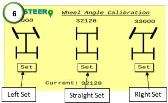
6) Calibrate the wheel angle sensor (WAS) limits. Ensure the current reading angle is not reading 0. Turn the steering wheel full lock left and press the left set button. Turn the wheel full lock right and press the right set button. Turn the wheel to dead straight and press the straight set button. Check the values above each set point to see if they've changed. Repeat the straight calibration using the WAS calibration procedure in step 9 on next page.
