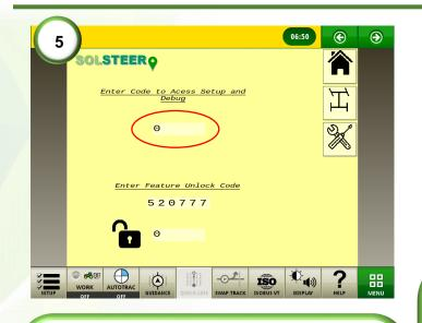
**5)** Access the setup and dealer lever diagnostics page. Enter the code 835 into the debug field.
