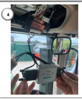
**4)** Connect the 29-way connector of the Fendt Vario MT Agri-Steer Interface Harness (7) to the 29-way connector that has been disconnected. Connect the D-sub connector labelled 'SCAN' (8) into the SCAN side of the Agri-Steer module and the D-sub connector labelled 'GCAN' (10) into the GCAN side of the module.
