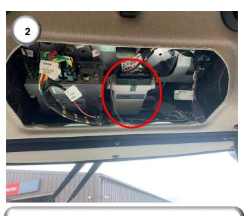
**2)** This will reveal the VD03 controller in the centre of the roof.
