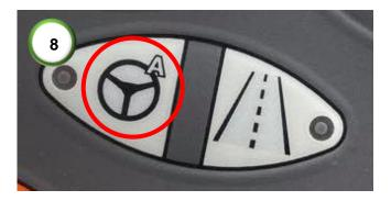
**8)** To engage, press the white steering engage button as shown. This can also be programmed to any button on the joystick via the Fendt Vario MT terminal. **Note:** Moving the steering wheel at any time will disengage.
