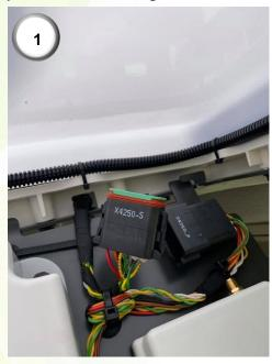
1) Locate and remove the inside roof panel where a standard receiver would be located. Mount the Agri-Steer here. Locate the two 12-way connectors and disconnect them.
