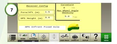
7) Ensure the receiver config settings are correct. Fore/Aft is the distance between the center of the fixed axle to the receiver. A TCM calibration will be required after changing these values. The maximum speed that the wheels can be turn can be set under 'Max Wheel Angle Velocity'. Default is 5°/sec.
