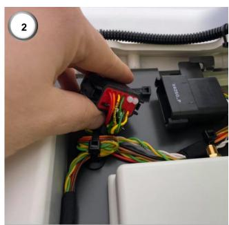
2) Connect the 12-way male connector plug to the 12-way female connector socket of the harness (9). Plug both D-Sub Connectors (10 and 12) into the Agri-Steer Module (11) with GCAN in the GCAN side and the SCAN in the SCAN side.
