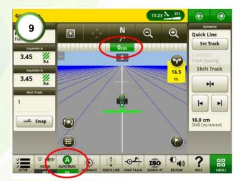
**9)** Engage the steering and drive at about 4kph. Wait for the cross-track error to be holding a stable value around 0cm.
