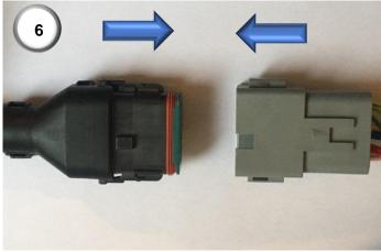
**5)** Plug in the male 9-pin from the GCAN adaptor harness (8) into the female 9-pin that has just been unscrewed from the panel. This enables the use of the ISO-joystick if needed.
