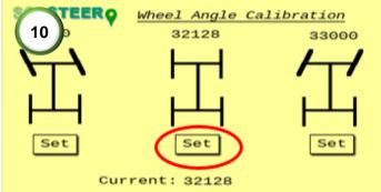
**10)** While tracking on-line, press the straight set button in the setup page. This will save the dead center point of the wheel angle sensor (WAS).
