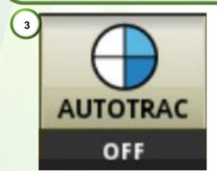
**3)** Once an A-B line is set, arm the GreenStar for steering. This is done by pressing the 'AUTOTRAC' button at the bottom of the screen. Once three-quarters of the circle are filled the system is ready to engage. **IMPORTANT!** Disarm the GreenStar steering.
