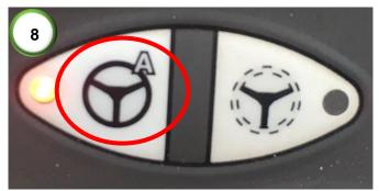
**8)** To engage, press the white steering engage button as shown. This can also be programmed to any button on the joystick via the FendtONE terminal. **Note:** Moving the steering wheel at any time will disengage.
