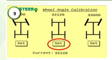
**9)** While tracking on-line, press the straight set button in the setup page. This will then save the dead center point of the wheel angle sensor (WAS).
