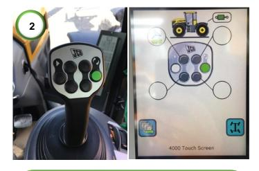
**2)** Assign the engage button to one of the buttons on the main control joystick.
