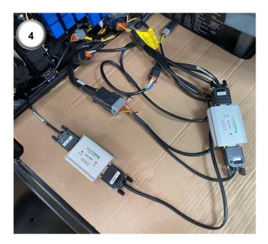
4) Plug in the D-sub connector labelled 'GCAN'
