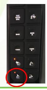
1) Turn the ignition on and press the GPS button on the panel. Wait for the GreenStar to turn on. Note that the LED's on the Agri-Steer module will be red until communication is made with the GreenStar display. The GreenStar will display 'Automatic steering detected' and the LED's will start flashing green when the system is ready to use.
