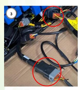
**3)** Plug the JCB/005 harness into the two 12way connectors using the two 12-way connectors of the harness (1 and 6).
