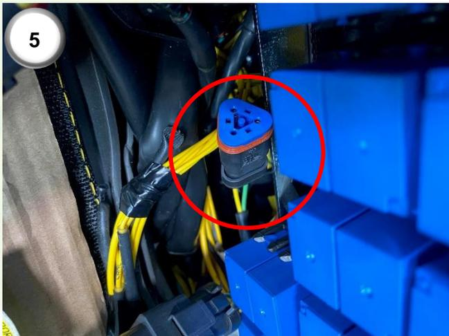
**5)** Also in the fuse cupboard locate the 3-way Deutsch male connector labelled 'Coverage'. Plug the 3-way female Deutsch connector (3) of the JCB/006 harness onto this connector.
