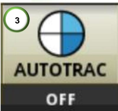
3) Once an A-B line is set, arm the GreenStar for steering. This is done by pressing the 'AUTOTRAC' button at the bottom of the screen. Once three-quarters of the circle are filled the system is ready to engage. **IMPORTANT!** Disarm the GreenStar steering with two-quarters of the circle full when travelling on public roads.
