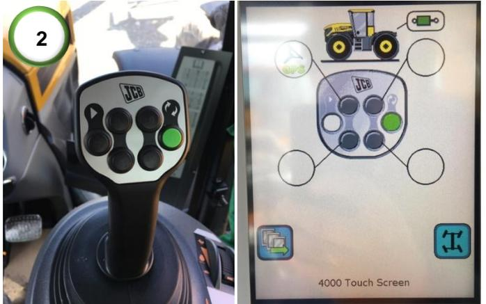
2) Assign the engage button to one of the buttons on the main control joystick.
