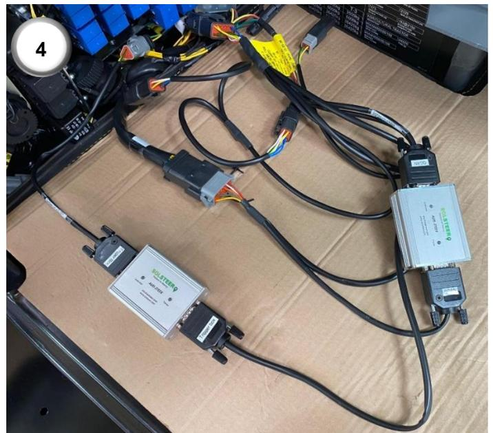
**4)** Plug in the D-sub connector labelled 'GCAN' (9) to the Greenstar side of the Agri-Steer Module (8). Plug in the D-sub connector labelled 'SCAN' (7) to the tractor side of the Agri-Steer module. Plug the D-sub connectors labelled 'Trigger Box' (4) into the trigger box (5).
