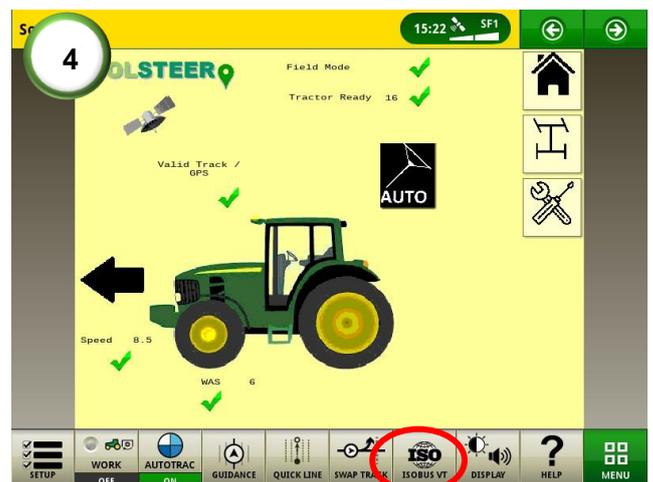
4) Locate the Solsteer page by clicking on the ISOBUS VT icon. When there is a valid track selected, a valid GPS signal and the vehicle is ready to engage, all pre-acquisitions should be ticked.
