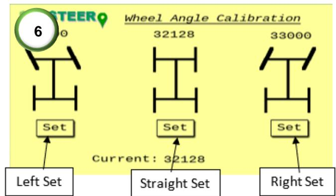
6) Calibrate the wheel angle sensor (WAS) limits. Ensure the current reading angle is not reading 0. Turn the steering wheel full lock left and press the left set button. Turn the wheel full lock right and press the right set button. Turn the wheel to dead straight and press the straight set button. Check the values above each set point to see if they've changed. Repeat the straight calibration using the WAS calibration procedure in step
