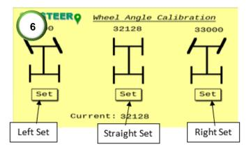
6) Calibrate the wheel angle sensor (WAS) limits. Ensure the current reading angle is not reading 0. Turn the steering wheel full lock left and press the left set button. Turn the wheel full lock right and press the right set button. Turn the wheel to dead straight and press the straight set button. Check the values above each set point to see if they've changed.
