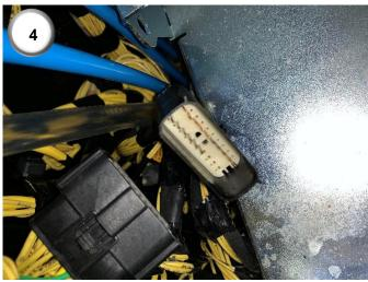
**4)** Split the two connectors. Plug in the 20-way Molex connector of the JCB 8000 Agri-steer interface harness (6). The other half will no longer be used.
