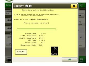
8) Move the wheel to the middle position and press either the engage button and or the black softkey engage button to start the calibration process. Follow the on-screen instructions, every step will require the engage button to be pressed to start. NOTE: The wheels will automatically move in this routine, ensure no-body is near the machine.
