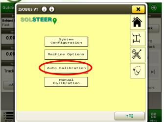
**7)** Press the 'Spanner and Screwdriver' button and go into 'Auto Calibration'.
