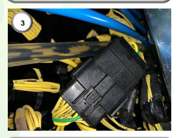
3) Locate the connector labelled 'GPS'.
