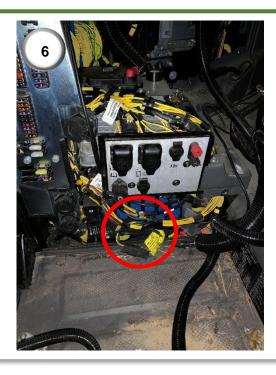
**6)** If the tractor has a factory fitted ISOBUS harness, split the 4-way connector and join in the 4-way connectors of the JCB 8000 Agri-steer harness (8 and 9).
