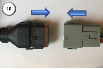
**10)** Connect the 12-way connector of the GS3 harness (5) to the 12-way connector of the JCB vehicle harness (10).
