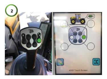
**2)** Assign the engage button to one of the buttons on the main control joystick. Recording triggers for the Hitch, SCV's and PTO are also available.
