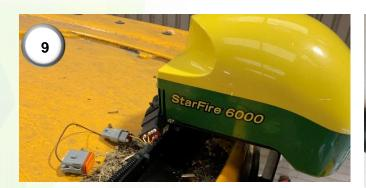
**9)** Connect the 12-way connector (2) to the StarFire receiver.
