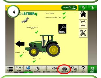
**4)** Locate the Solsteer page by clicking on the ISOBUS VT icon. When there is a valid track selected, a valid GPS signal and the vehicle is ready to engage, all pre-acquisitions should be ticked.
