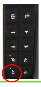
1) Turn the ignition on and press the GPS button on the panel. Wait for the GreenStar to turn on. Note that the LED's on the Agri-Steer module will be red until communication is made with the GreenStar display. The GreenStar will display 'Automatic steering detected' and the LED's will start flashing green when the system is ready to use.
