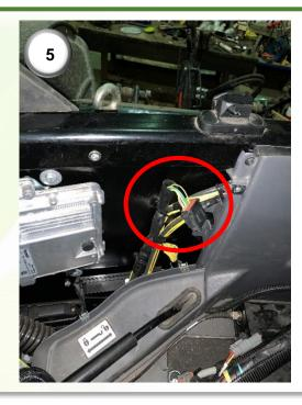
**5)** Connect the 12-way mini Deutsch connector of the JCB 8000 Agri-steer harness (11) to the 12-way mini Deutsch connector labelled 'coverage' at the back of the cab.
