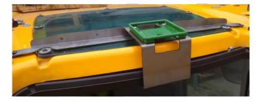
7) To run the GS3 harness to the Starfire, remove the black panel that holds the A/C and the radio. Remove the pins the 12-way connector to allow the harness to be pushed through holes. Remove the right-hand speaker to make it easier to push the rubber grommet. Drop the front right exterior work lights and push the harness through.
