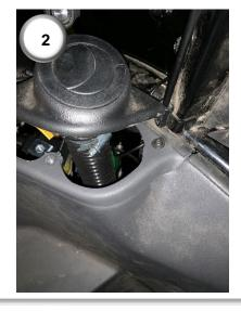
1) Locate the right-hand console panel. Remove the panel by removing 13 bolts. **2)** This includes two hidden bolts under the plastic air vent holder.
