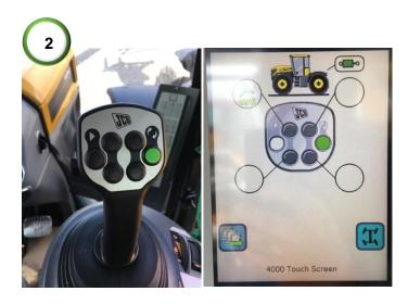
**2)** Assign the engage button to one of the buttons on the main control joystick. Recording triggers for the Hitch, SPV's and PTO are also available.
