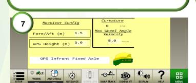
7) Ensure the receiver config settings are correct. Fore/Aft is the distance between the center of the fixed axle to the receiver. A TCM calibration will be required after changing these values. The maximum speed that the wheels can be turn can be set under 'Max Wheel Angle Velocity'. Default is 5°/sec.
