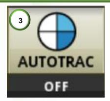
3) Once an A-B line is set, arm the GreenStar for steering. This is done by pressing the 'AUTOTRAC' button at the bottom of the screen. Once three-quarters of the circle are filled the system is ready to engage. IMPORTANT! Disarm the GreenStar steering with two-quarters of the circle full when travelling on public roads.
