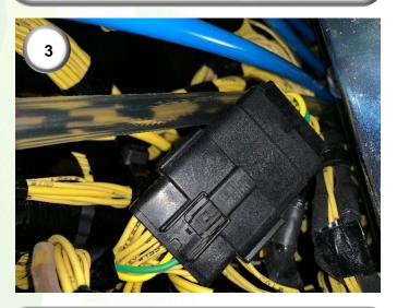
3) Locate the connector labelled 'GPS'.
