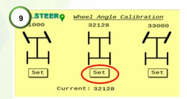
**9)** While tracking on-line, press the straight set button in the setup page. This will then save the dead center point of the wheel angle sensor (WAS).
