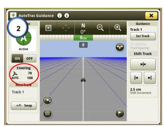
**2)** Select the steering icon shown. On the menu select 'steering adjustments. The following options can be adjusted.
