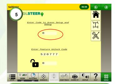
**5)** Access the setup and dealer lever diagnostics page. Enter the code 835 into the debug field.
