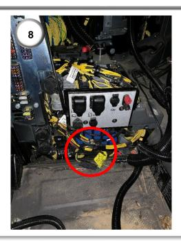
8) If the tractor has a factory fitted ISOBUS harness, split the 4-way connector and join in the male 4-way connector (10) and the female 4-way connector (11) of the Agri-Steer harness.
