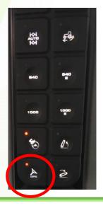
1) Turn the ignition on and press the GPS button on the panel. Wait for the GreenStar to turn on. Note that the LED's on the Agri-Steer module will be red until communication is made with the GreenStar display. The GreenStar will display 'Automatic steering detected' and the LED's will start flashing green when the system is ready to use.
