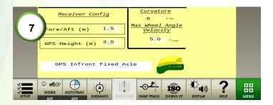
7) Ensure the receiver config settings are correct. Fore/Aft is the distance between the center of the fixed axle to the receiver. A TCM calibration will be required after changing these values. The maximum speed that the wheels can be turn can be set under 'Max Wheel Angle Velocity'. Default is 5°/sec.
