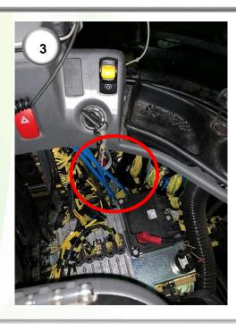
3) Locate the connector labelled 'GPS'.
