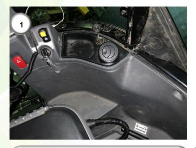
1) Locate the right-hand console panel. Remove the panel by removing 13 bolts.
