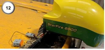
**12)** Connect the 12-way connector (2) to the StarFire receiver.
