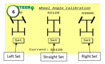
6) Calibrate the wheel angle sensor (WAS) limits. Ensure the current reading angle is not reading 0. Turn the steering wheel full lock left and press the left set button. Turn the wheel full lock right and press the right set button. Turn the wheel to dead straight and press the straight set button. Check the values above each set point to see if they've changed. Repeat the straight calibration using the WAS calibration procedure in step 8.
