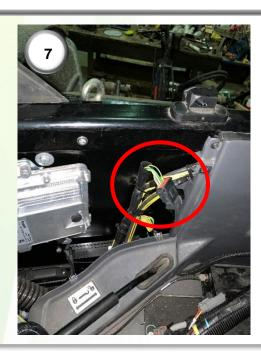
**7)** Connect the connector labelled 'coverage' to the 12-way connector at the back of the cab (7).
