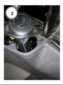
**2)** This includes two hidden bolts under the plastic air vent holder.
