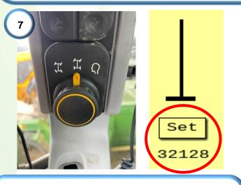
**7)** To calibrate the straight lock position, lift and twist the knob on the upright pillar in the cab. This will lock the rear wheels in position. Turn the front wheels to the straight position and press the 'Set' button.
