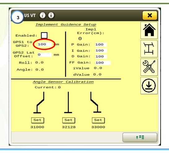
**3)** Measure the distance between the machine receiver and the implement receiver. Enter the value into the 'GPS1 to GPS2' box. Tick the 'Enabled' tickbox to active implement steering.
