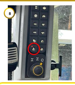
**8)** Ensure that the 'GPS' button is enabled, ready for auto-steering.
