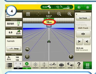
**4)** Lock the rear axle of the machine and engage the steering. Record the value of the implement receiver cross track error.
