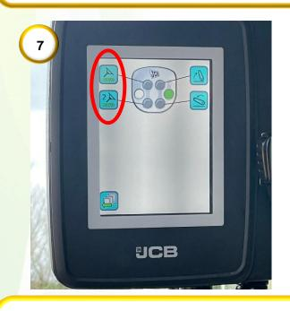
**7)** If using 'manual' mode, check the two buttons on the left are set up on 'AUTO' for front wheel engagement and rear wheel engagement. If using 'auto' mode check that only the top left button has been assigned to 'AUTO'.
