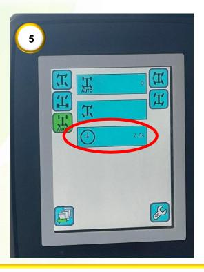
**5)** If using 'auto engage' mode, set the time period between the front wheels engaging and the rear wheels engaging.
