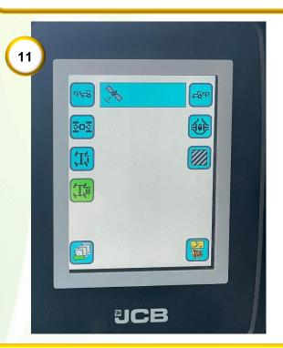
**11)** Ensure that the satellite icon is shown, and is **not** ticked, otherwise the rear axle will lock automatically upon engagement.
