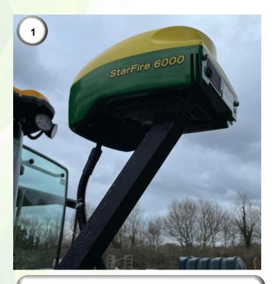
**1)** Mount the StarFire receiver behind the rear axle (bracket is not supplied).
