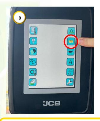
**9)** Press the icon shown. This step is to ensure that the rear axle will not lock upon auto-steer engagement.
