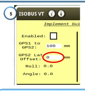
**5)** Return to the Solsteer VT page. Enter the value into the box shown, making sure it is the **negative** version of the value. For example for a cross track error of 10cm enter **-100mm** into the box.
