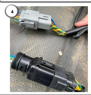
**4)** Tee into the two 12-way connectors with the JCB Rear Receiver Adaptor harness.
