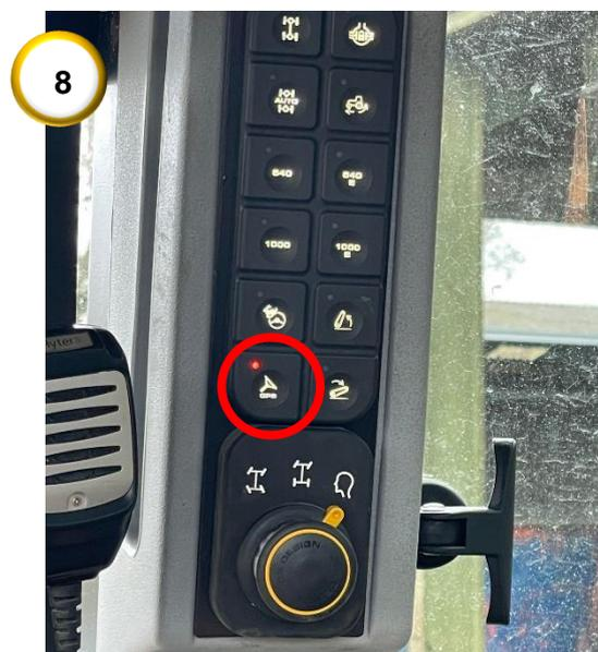
**8)** Ensure that the 'GPS' button is enabled, ready for auto-steering.
