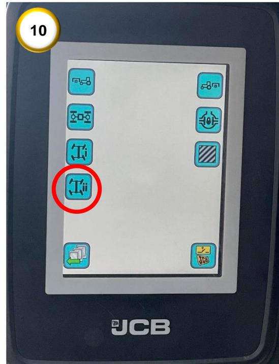
9) Press the icon shown. This step is to ensure that the rear axle will not lock upon auto-steer engagement.
