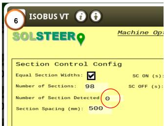
**5)** Enter the number of individual sections that are needed to be controlled. Enter the section spacing in mm.
