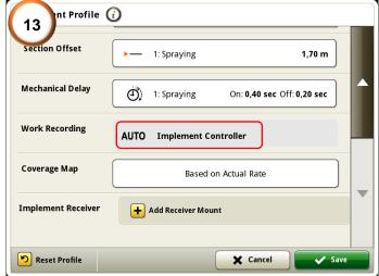
**12)** Ensure that all the working width, dimensions and section offset are all populated correctly. The tractor and sprayer profiles should be completed by the operator. Defaults are set from factory; however these could vary from machine to machine.
