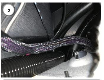
**2)** Locate the large diameter conduit. This runs from the back right-hand corner of the cab to the front middle section outside the cab.
