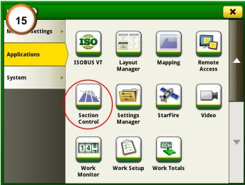
**14)** Select the work recording to be set to 'Section Control'.
