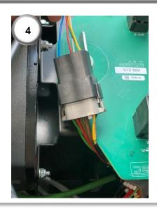
4) Lift the cover under the armrest. Lift the fuse board up and locate the grey male Deutsch 12-way connector, this should be labelled 'GPS'. Note: there might be a connector already connected if there has been another GPS system installed. If so, then disconnect it. Connect the Agri-steer in here, using the Deutsch 12-way socket labelled 'GPS' (7).
