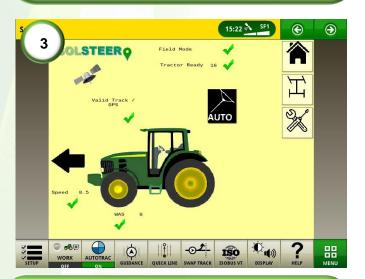
**3)** When there is a valid track is selected, a valid GPS signal and the vehicle is ready to engage, all pre-acquisitions should be ticked.
