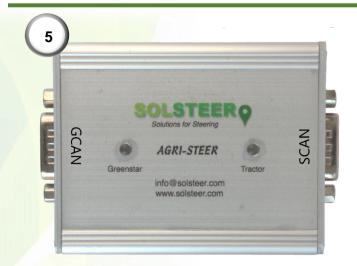
5) Plug in the D-Sub connector labelled 'GCAN' (9) to the Greenstar side of the Agri-steer module. Plug in the D-Sub connector labelled 'SCAN' (8) to the tractor side of the Agri-steer module. Connect the GS3 harness to the Agri-Fac harness adaptor using the two 12-way Deutsch connectors (3 and 4).
