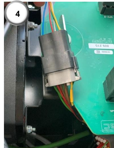
**4)** Lift the cover under the armrest. Lift the fuse board up and locate the grey male Deutsch 12-way connector, this should be labelled 'GPS'. Note: there might be a connector already connected if there has been another GPS system installed. If so, then disconnect it. Connect the Agri-steer in here, using the Deutsch 12-way socket labelled 'GPS' (7).
