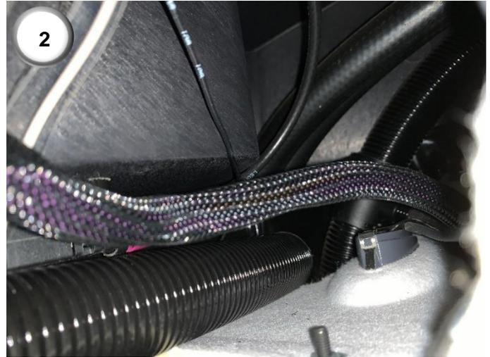
**2)** Locate the large diameter conduit. This runs from the back right-hand corner of the cab to the front middle section outside the cab.
