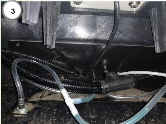
**3)** Drop the front black light section down at the front of the cab. This reveals the other end of the conduit. Remove the 12-way connector plug (3) of the GS3 harness. Thread the harness from the cab, through the conduit and to the outside of the cab. Using the diagram on page 12, reinstall the 12-way connector plug of the GS3 with the pinouts shown. Connect the 12-way connector to the Starfire receiver.
