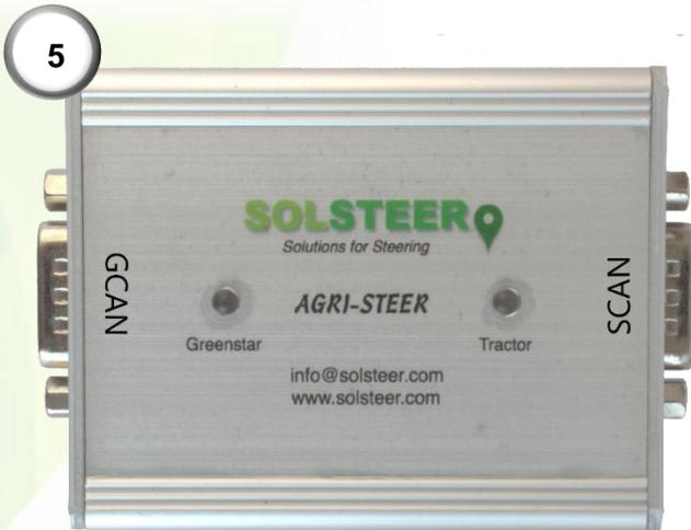
**5)** Plug in the D-Sub connector labelled 'GCAN' (9) to the Greenstar side of the Agri-steer module. Plug in the D-Sub connector labelled 'SCAN' (8) to the tractor side of the Agri-steer module. Connect the GS3 harness to the Agri-Fac harness adaptor using the two 12-way Deutsch connectors (3 and 4).
