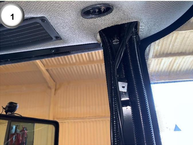
**1)** To install the GS3 harness, remove the plastic cover on the back right-hand cab upright. Remove the right-hand side switch panel on the roof.
