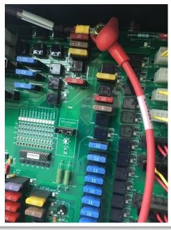
2) There is no permanent power in the 9-way ISO socket. Therefore run the power lead with the fuse down into the fuse box. Locate the red positive bolt and attach it here. Remove the roof panel on top of the roof and run the receiver cable up the cab upright.
