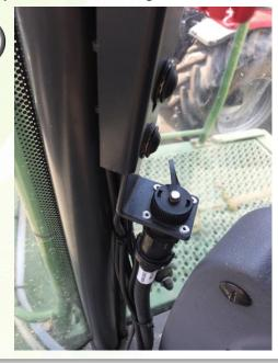
1) Locate the 9-way ISO socket inside the cab. This is usually on the front right cab up-right. Plug in the Agri-steer harness in here using the 9-wawy ISOBUS plug (8).
