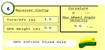
6) Ensure the receiver config settings are correct. Fore/Aft is the distance between the center of the fixed axle to the receiver. A TCM calibration will be required after changing these values. The maximum speed that the wheels can be turn can be set under 'Max Wheel Angle Velocity'. Default is 5°/sec.
