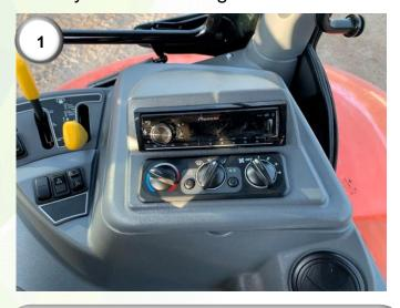
1) Lift the housing that holds the radio and A/C controls. Locate the fuse board under the black cover.
