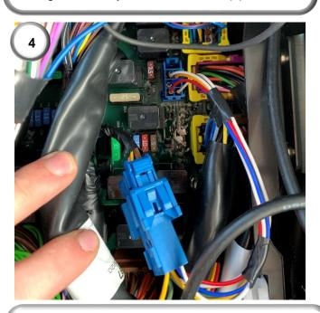
**4)** 'Tee' into the two 6-way connectors in the cab using the in-cab 6 way connectors of the Kubota harness (9 and 10).
