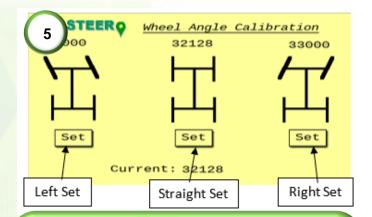
5) Calibrate the wheel angle sensor (WAS) limits. Ensure the current reading angle is not reading 0. Turn the steering wheel full lock left and press the left set button. Turn the wheel full lock right and press the right set button. Turn the wheel to dead straight and press the straight set button. Check the values above each set point to see if they have changed. Repeat the straight calibration using the WAS calibration procedure in step 8.
