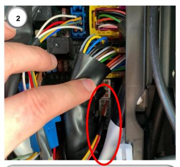
2) Locate the white 14-way Molex connector on the fuse board. This is usually found in the bottom right hand corner and is labelled 'GPS'. Connect the Kubota interface harness here using the 14-way Molex connector (7).
