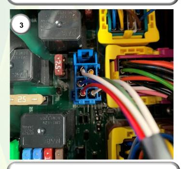
**3)** Locate the blue 6-way connector which has 'ISOBUS' printed on the board. Disconnect the connector that is already connected.
