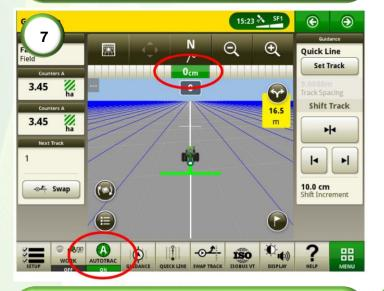
**7)** Engage the steering and drive at about 4kph. Wait for the cross-track error to be holding a stable value around 0cm.
