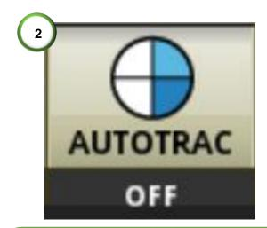
2) Once an A-B line is set, arm the GreenStar for steering. This is done by pressing the 'AUTOTRAC' button at the bottom of the screen. Once three-quarters of the circle are filled the system is ready to engage.
