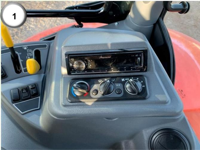
**1)** Lift the housing that holds the radio and A/C controls. Locate the fuse board under the black cover.
