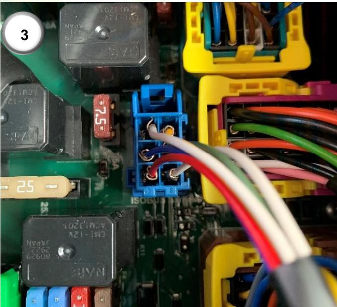
**3)** Locate the blue 6-way connector which has 'ISOBUS' printed on the board. Disconnect the connector that is already connected.
