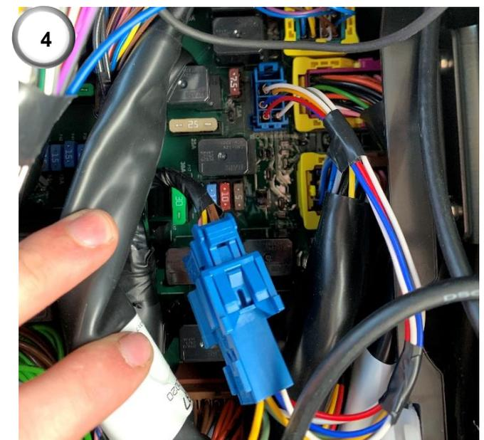
**4)** 'Tee' into the two 6-way connectors in the cab using the in-cab 6 way connectors of the Kubota harness (9 and 10).
