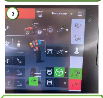
**3)** Set the engage button to a button on the main control joystick.
