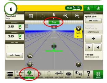
**8)** Engage the steering and drive at about 4kph. Wait for the cross-track error to be holding a stable value around 0cm.
