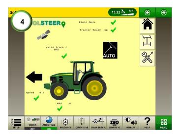
**4)** When there is a valid track is selected, a valid GPS signal and the vehicle is ready to engage, all pre-acquisitions should be ticked.
