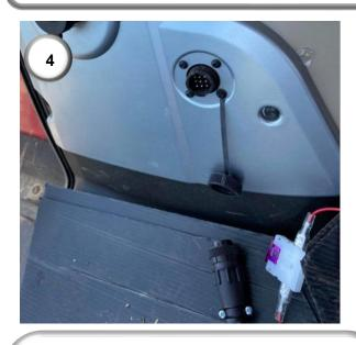
3) Connect the StarFire roof harness by connecting the 12-way female connector (3) to the connector on the roof. Connect the Deutsch 12-way Connector Socket to the StarFire receiver. Mount the StarFire receiver as far forward and as central as possible.
