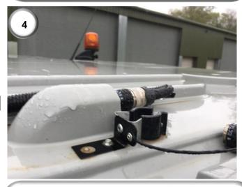
**4)** Connect the StarFire roof harness by connecting the 12-way female connector (3) to the connector on the roof. Connect the Deutsch 12-way Connector Socket to the StarFire receiver. Mount the StarFire receiver as far forward and as central as possible.
