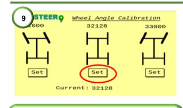
**9)** While tracking on-line, press the straight set button in the setup page. This will then save the dead center point of the wheel angle sensor (WAS).
