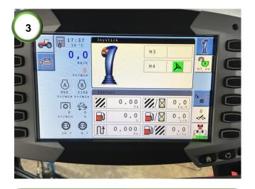
**3)** Set the engage button to a button on the main control joystick.
