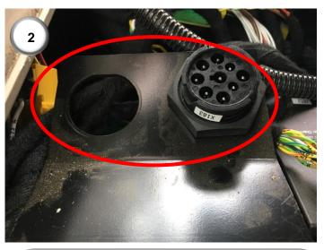
2) Connect the GCAN 9-way Connector (11) of the GCAN adaptor (10) to the connector labelled 'X183' in the cab. Connect the SCAN 9-way Connector (16) of the GCAN adaptor (14) to the connector labelled 'X184' in the cab. To make room for the panel to be replaced, undo the plastic nut and secure connectors elsewhere.
