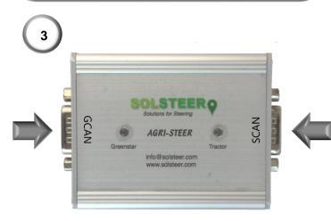
**3)** Connect the GCAN and SCAN D-Sub connectors (12 and 14 respectively) to the Agri-Steer module (13), into the corresponding ports labelled 'GCAN' and 'SCAN'.
