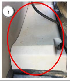
**1)** Locate and remove the fuse panel on the right-hand side of the cab, next to the seat.
