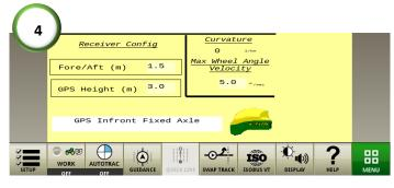
**5)** Ensure the receiver config settings are correct. Fore/Aft is the distance between the center of the fixed axle to the receiver. The maximum speed that the wheels can be turn can be set under 'Max Wheel Angle Velocity'. Default is 5°/sec. Check under the spanner and screwdriver that the swather is selected.
