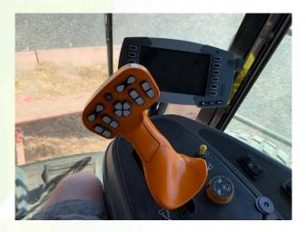
To engage the steering by pressing the auto engage button on the joystick. NOTE: The swather will only engage if 1<sup>st</sup> gear is selected.
