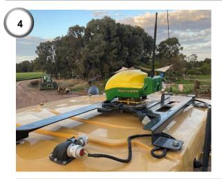
**4)** Connect the Roof Harness by connecting the 30-way female connector (4) to the connector on the roof. Connect the Deutsch 12-way Connector Socket to the StarFire receiver. Mount the StarFire receiver as far forward and as central as possible.
