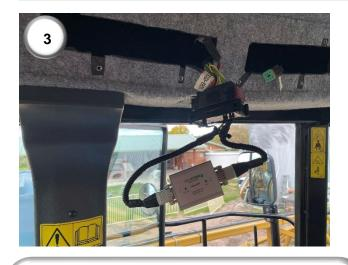
**3)** Connect the GCAN and SCAN connectors of the A/017 harness (6 and 8) to the Solsteer Agri-Steer. Connect the two 29-way connectors together (5).
