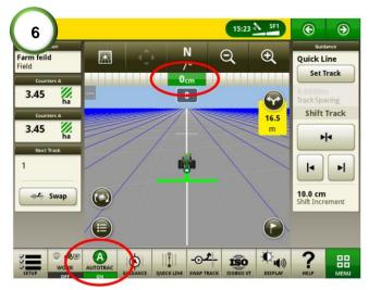
**6)** Engage the steering and drive at about 4kph. Wait for the cross-track error to be holding a stable value around 0cm.
