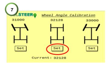
**7)** While tracking on-line, press the straight set button in the setup page. This will then save the dead center point of the wheel angle sensor (WAS).
