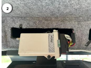
**1)** Above the drivers seat locate the panel containing the white controller box.
