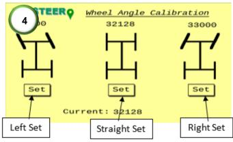
4) Calibrate the wheel angle sensor (WAS) limits. Ensure the current reading angle is not reading 0. Turn the steering wheel full lock left and press the left set button. Turn the wheel full lock right and press the right set button. Turn the wheel to dead straight and press the straight set button. Check the values above each set point to see if they've changed. Repeat the straight calibration using the WAS calibration procedure in step 8.
