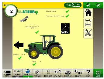
1) Turn the ignition on and wait for the GreenStar to turn on. Note that the LED's on the Agri-Steer module will be red until communication is made with the GreenStar display.
