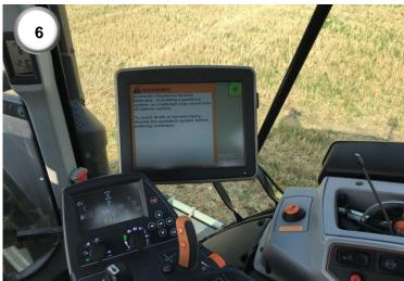
**5)** Connect the 9-way ISOBUS socket (9) of the display cab harness to the ISOBUS port in the cab, next to the unlock lever for the hitch. Connect the red wire coming out of the display harness to a permanent positive power supply.
