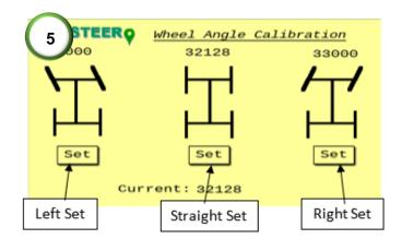
5) Calibrate the wheel angle sensor (WAS) limits. Ensure the current reading angle is not reading 0. Turn the steering wheel full lock left and press the left set button. Turn the wheel full lock right and press the right set button. Turn the wheel to dead straight and press the straight set button. Check the values above each set point to see if they've changed. Repeat the straight calibration using the WAS calibration procedure in step 8.
