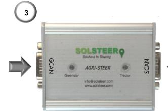
**3)** Connect the GCAN and SCAN D-Sub connectors (11 and 13 respectively) to the Agri-Steer module (12), into the corresponding ports labelled 'GCAN' and 'SCAN'.
