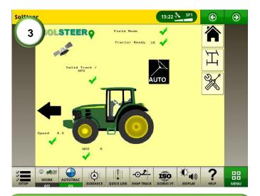
**3)** When there is a valid track is selected, a valid GPS signal and the vehicle is ready to engage, all pre-acquisitions should be ticked.
