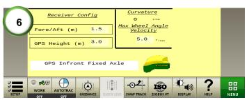
6) Ensure the receiver config settings are correct. Fore/Aft is the distance between the center of the fixed axle to the receiver. A TCM calibration will be required after changing these values. The maximum speed that the wheels can be turn can be set under 'Max Wheel Angle Velocity'. Default is 5°/sec.
