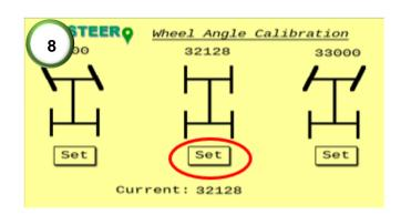
**8)** While tracking on-line, press the straight set button in the setup page. This will then save the dead center point of the wheel angle sensor (WAS).
