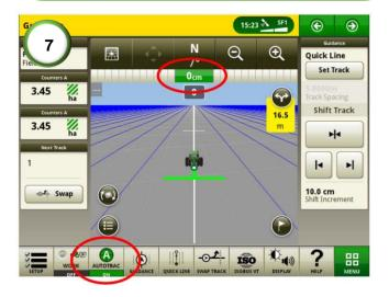
**7)** Engage the steering and drive at about 4kph. Wait for the cross-track error to be holding a stable value around 0cm.
