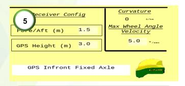
5) Ensure the receiver config settings are correct. Fore/Aft is the distance between the center of the fixed axle to the receiver. A TCM calibration will be required after changing these values. The maximum speed that the wheels can be turn can be set under 'Max Wheel Angle Velocity'. Default is 5°/sec.
