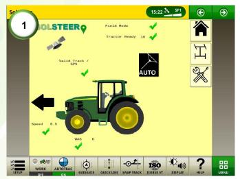
1) Turn the ignition on and wait for the GreenStar to turn on. Locate the SolSteer page by clicking on the ISOBUS VT icon. When there is a valid track selected, a valid GPS signal and the vehicle is ready to engage, all pre-acquisitions should be ticked.
