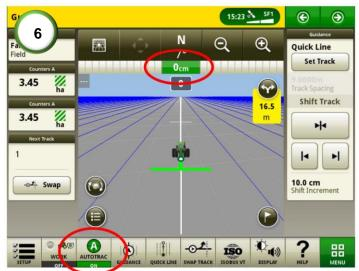
**6)** Engage the steering and drive at about 4kph. Wait for the cross-track error to be holding a stable value around 0cm.
