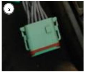
1) Remove the grey panel behind the cab seat and find the 12-way Deutsch connection labelled 'Armrest'. Split the connection and insert the 12-way male and female connectors (8 and 9) of the Versatile Agri-steer inside cab harness
