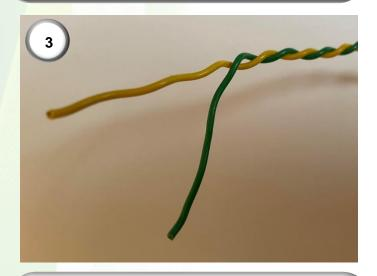
3) If connection to an ISOBUS harness is required, there are yellow and green CANBUS tails near the green 12-way Deutsch connector in the cab (Yellow = CAN High, Green=CAN Low).
