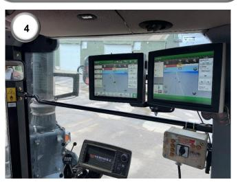
4) Run the display cable to the display and mount the Greenstar screen. Connect the 26-way Connector Plug (2) into the display. Connect the Versatile Agri-Steer inside cab harness to the ECU using the 46-way Molex connector.
