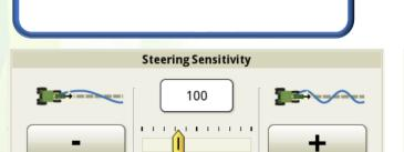
3) Adjust this parameter to make the system more aggressive. The higher this number, the more the wheels will turn for the same amount of error.
