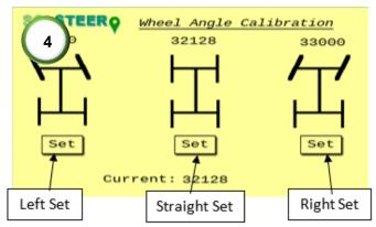
4) Calibrate the wheel angle sensor (WAS) limits. Ensure the current reading angle is not reading 0. Turn the steering wheel full lock left and press the left set button. Turn the wheel full lock right and press the right set button. Turn the wheel to dead straight and press the straight set button. Check the values above each set point to see if they have changed. Repeat the straight calibration using the WAS calibration procedure in step 8.
