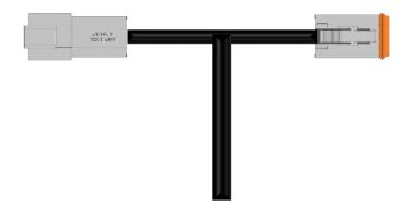
8) Follow the cable from the wheel angle sensor back towards the cab until the 3-way Deutsch connector is found. 'T' in the 3-way connectors on the outside harness here. This will access the WAS signal. Route the receiver harness up the cab and along to the receiver.
