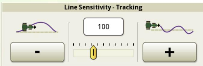
**5)** If the machine moves too far from the A-B line increase the tracking line sensitivity. If the machine is unstable on AB line decrease this value.
