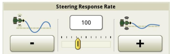
**8)** If the tracking performance is poor due to the system being too slow, increase the steering response rate. Increasing this too much, can result in jittery behavior.
