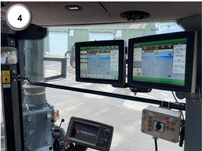
**4)** Run the display cable to the display and mount the Greenstar screen. Connect the 26-way Connector Plug (2) into the display. Connect the Versatile Agri-Steer inside cab harness to the ECU using the 46-way Molex connector.
