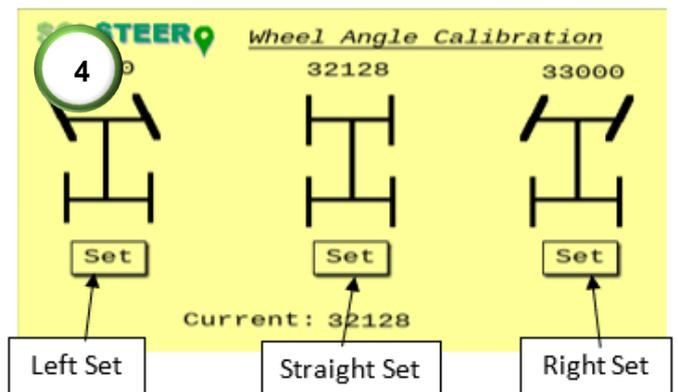
4) Calibrate the wheel angle sensor (WAS) limits. Ensure the current reading angle is not reading 0. Turn the steering wheel full lock left and press the left set button. Turn the wheel full lock right and press the right set button. Turn the wheel to dead straight and press the straight set button. Check the values above each set point to see if they have changed. Repeat the straight calibration using the WAS calibration procedure in step 8.
