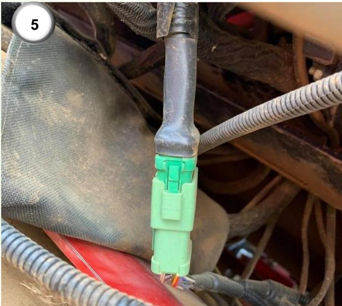
**5)** Locate the Green 12-way connector outside the cab. This is found on the right of the machine, under the cab, in between the pivot point. Connect the outside harness here using the 12-way green Deutsch connector (10) of the Versatile Agri-Steer outside harness.
