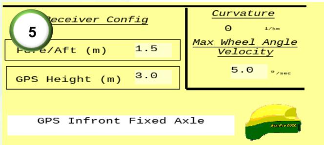
5) Ensure the receiver config settings are correct. Fore/Aft is the distance between the center of the fixed axle to the receiver. A TCM calibration will be required after changing these values. The maximum speed that the wheels can be turn can be set under 'Max Wheel Angle Velocity'. Default is 5°/sec.
