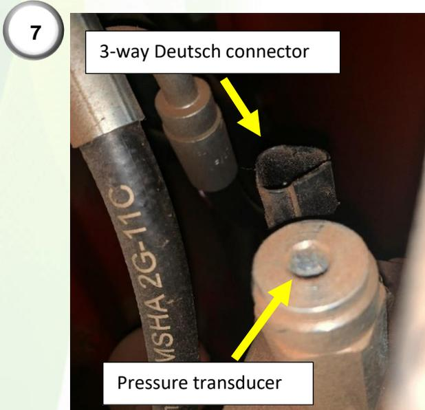
**7)** Connect the 3-way Deutsch connector plug from the outside harness (12) onto the pressure transducer. This is found on the back of the valve.
