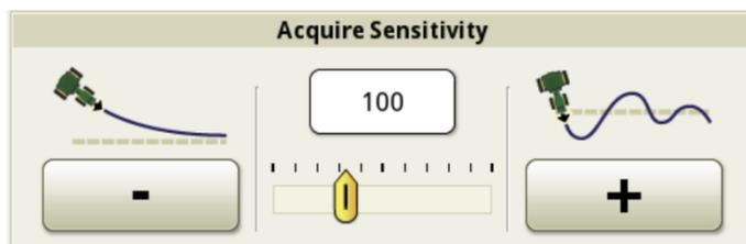
4) Adjust this parameter until the acquisition is satisfactory. The higher this number, the more aggressive the vehicle will turn onto the line.
