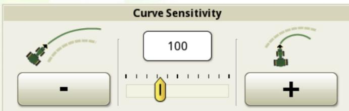
**9)** This parameter adjusts how sensitive the system is to curves on the track. The higher the number the more the vehicle will undercut the line. Adjust this to improve the tracking performance when driving around a curve.
