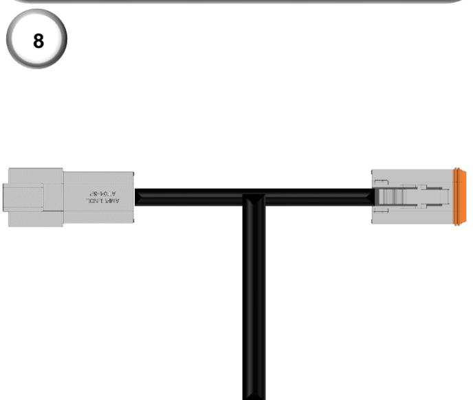
**8)** Follow the cable from the wheel angle sensor back towards the cab until the 3-way Deutsch connector is found. 'T' in the 3-way connectors on the outside harness here. This will access the WAS signal. Route the receiver harness up the cab and along to the receiver.
