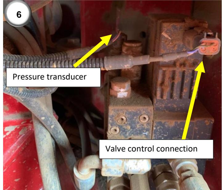
**6)** Locate the steering valve block, this is found under the cab on the right of the machine. Connect the Deutsch 4-way plug of the Versatile Agri-Steer outside harness (13) to the 4-way Deutsch on the valve. The connector is usually unused if no steering is installed on the machine.
