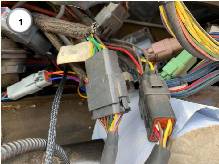
**1)** Remove the grey panel behind the cab seat and find the 12-way Deutsch connection labelled 'Armrest'. Split the connection and insert the 12-way male and female connectors (8 and 9) of the Versatile Agri-steer inside cab harness
