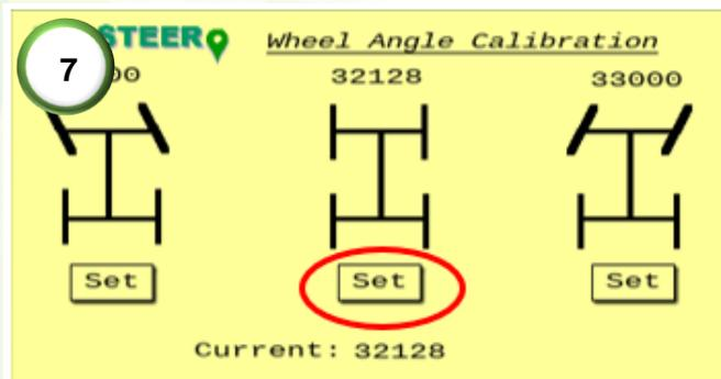
7) While tracking on-line, press the straight set button in the setup page. This will then save the dead center point of the wheel angle sensor (WAS).
