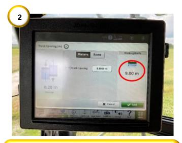
2) Change the header width on the Cebis terminal and ensure the width also changes on the GreenStar.
