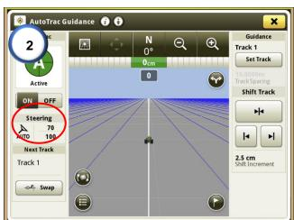
**2)** Select the steering icon shown. On the menu select 'steering adjustments'. The following options can be adjusted.
