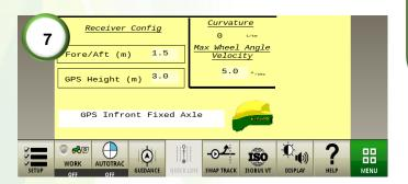
7) Ensure the receiver config settings are correct. Fore/Aft is the distance between the center of the fixed axle to the receiver. A TCM calibration will be required after changing these values. The maximum speed that the wheels can be turn can be set under 'Max Wheel Angle Velocity'. Default is 5°/sec.
