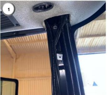
1) To install the GS4, remove the plastic cover on the back-right cab upright. Remove the right-hand switch panel on the roof.
