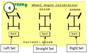
6) Calibrate the wheel angle sensor (WAS) limits. Ensure the current reading angle is not reading 0. Turn the steering wheel full lock left and press the left set button. Turn the wheel full lock right and press the right set button. Turn the wheel to dead straight and press the straight set button. Check the values above each set point to see if they've changed. Repeat the straight calibration using the WAS calibration procedure in step 9.
