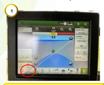
1) When the GreenStar is running, ensure the recording trigger has gone to 'AUTO'.
