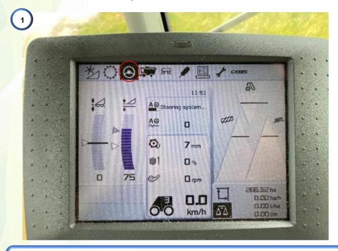
1) Use the black rotary knob to select the steering wheel icon. Select 'active guide sensor'. Select 'third party steering interface'. This can also be shown as 'Steering system from other manufacturer'.\*
