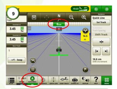
**9)** Engage the steering and drive at about 4kph. Wait for the cross-track error to be holding a stable value around 0cm.
