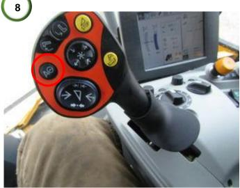
**8)** Engage the steering by pressing the 'auto' button shown (Note: cab interface and joystick may differ from the image shown).
