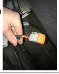
3) Remove the necessary panels and lights to gain access behind the 'Lexion' (between the top of the windscreen and below where the StarFire receiver would sit) section at the front of the cab. This reveals the outer end of the conduit. Remove the 12-way connector (2) of the GS4 harness. Thread the harness from the cab, through the conduit, and to the outside of the cab. Reinstall the 12-way connector. Pinouts are found on page 13.
