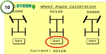
**10)** While tracking on-line, press the straight set button in the setup page. This will then save the dead center point of the wheel angle sensor (WAS).
