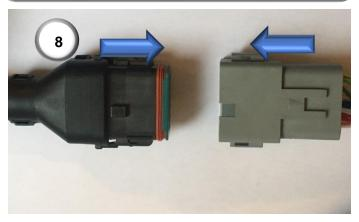
**8)** Join the 12-way Connector Socket on the GCAN adapter harness (6) to the 12-way Connector Plug on the GS3 harness (5). Fit the harness to the roof ready to connect to the StarFire receiver (2).
