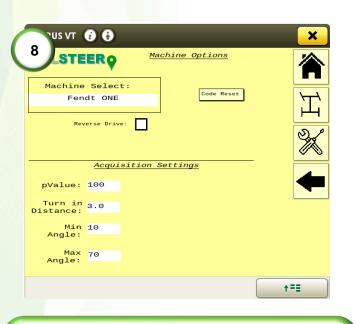
8) If machine alarm sounds, power off machine, disconnect SCAN plug from ECU/001, power on machine, Using debug code 835 (4) ensure <u>Machine Select</u>: is set to <u>Fendt ONE</u>. Perform another power cycle and alarm will not sound.
