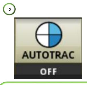
3) Once an A-B line is set, arm the GreenStar for steering. This is done by pressing the 'AUTOTRAC' button at the bottom of the screen. Once three-quarters of the circle are filled the system is ready to engage.
