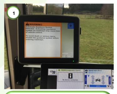
1) Turn the ignition on and wait for the GreenStar to turn on. Note that the LED's on the Agri-Steer module will be red until communication is made with the GreenStar display. The GreenStar will display 'Automatic Guidance System' warning and the LED's will start flashing green when the system is ready to use.
