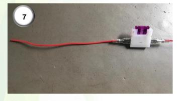
**7)** Connect the red wire to a unswitched 12v + source. This will ensure the GreenStar systems shuts down correctly.
