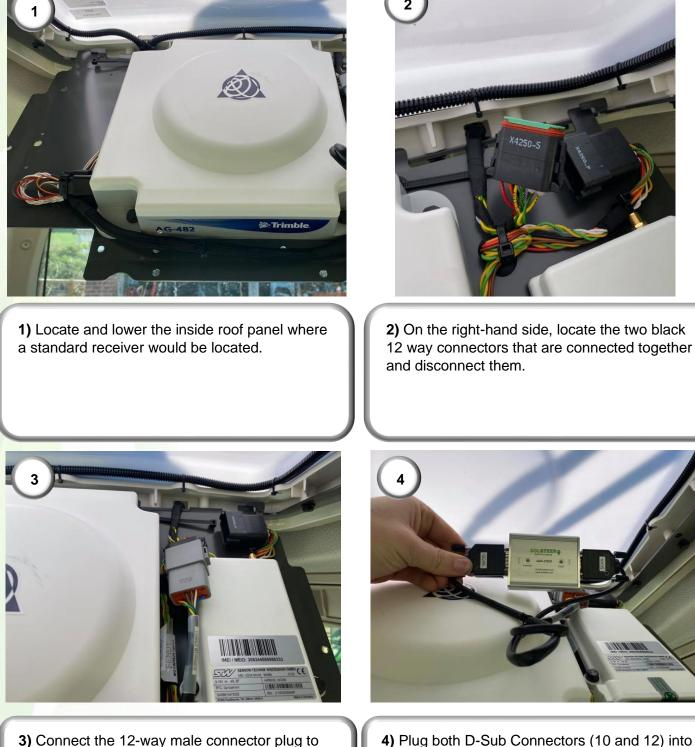
the 12-way female connector socket of the FendtONE SCAN adaptor (9).
