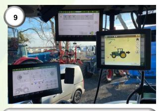
**9)** Mount the Greenstar Display (3) and connect the 26-way Connector plug (4) of the GS3 loom to the Greenstar Display in the 'Main' or 'Machine' socket.
