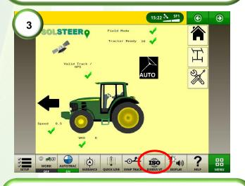
**3)** Locate the Solsteer page by clicking on the ISOBUS VT icon. When there is a valid track selected, a valid GPS signal and the vehicle is ready to engage, all pre-acquisitions should be ticked.
