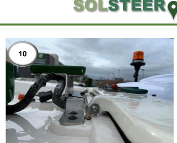
**10)** Mount the Fendt bracket on the roof of the machine. Mount the StarFire receiver on the roof as far forward and as central as possible. Run the StarFire cable with the 12- Way connector socket (2) along the roof and tighten it securely to the tractor. Join the connector to the StarFire receiver.
