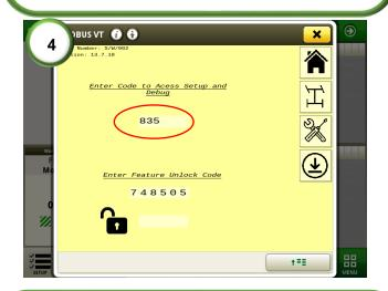
**4)** Access the setup and dealer lever diagnostics page. Enter the code **<u>835</u>** into the debug field.
