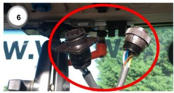
**5)** Locate the roof panel at the back of the cab and remove the screws holding it in place. Remove the two bolts holding the incab 9-way ISO connector and remove it from the hole.
