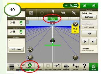
**10)** When calibration is complete, engage the steering and drive at about 4kph. Wait for the cross-track error to be holding a stable value around 0cm.
