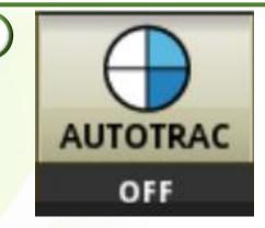
**4)** Once an A-B line is set, arm the GreenStar for steering. This is done by pressing the 'AUTOTRAC' button at the bottom of the screen. Once three-quarters of the circle are filled the system is ready to engage. **IMPORTANT!** Disarm the GreenStar steering with two-quarters of the circle full when travelling on public roads.
