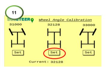
**11)** While tracking on-line, press the straight set button in the setup page. This will then save the dead center point of the wheel angle sensor (WAS).
