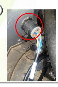
**1)** Locate the 47 way (female) connector behind the seat below the diagnostic socket. Remove any existing harness and Plug in the JCB/012 harness. (1)
