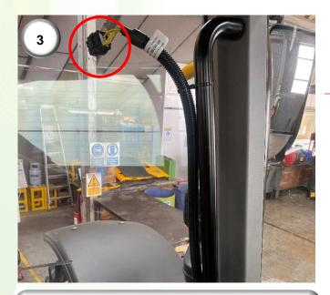
**3)** Plug the JCB 'Interface Ready' harness into your mounted GreenStar Display.
