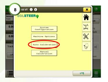
**8)** Press the 'Spanner and Screwdriver' button and go into 'Auto Calibration'.
