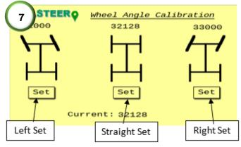
7) Calibrate the wheel angle sensor (WAS) limits. Ensure the current reading angle is not reading 0. Turn the steering wheel full lock left and press the left set button. Turn the wheel full lock right and press the right set button. Turn the wheel to dead straight and press the straight set button. Check the values above each set point to see if they've changed. Repeat the straight calibration
