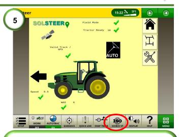
**5)** Locate the Solsteer page by clicking on the ISOBUS VT icon. When there is a valid track selected, a valid GPS signal and the vehicle is ready to engage, all pre-acquisitions should be ticked.
