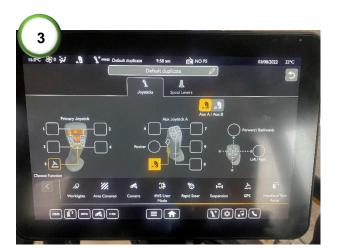
**3)** Assign the engage button to one of the buttons on the main control joystick.
