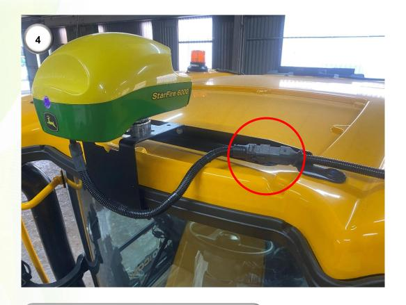
**4)** Plug your StarFire Receiver into the 'Interface ready' harness on the roof.
