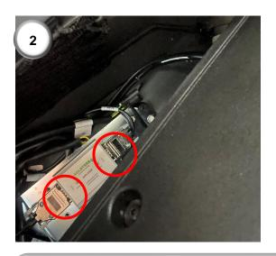
2) Connect the Agri-Steer module (ECU/001) to remaining D-subs as shown on the previous diagram (page 12).
