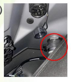
1) Locate the 47 way (female) connector behind the seat below the diagnostic socket. Remove any existing harness and Plug in the JCB/013 harness.
