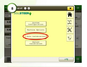
**8)** Press the 'Spanner and Screwdriver' button and go into 'Auto Calibration'.
