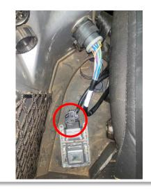
2) Connect the Agri-Steer module (ECU/002) to Molex 46 – way connector plug as shown on the previous diagram
