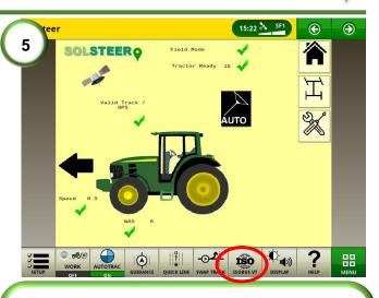
**5)** Locate the Solsteer page by clicking on the ISOBUS VT icon. When there is a valid track selected, a valid GPS signal and the vehicle is ready to engage, all pre-acquisitions should be ticked.
