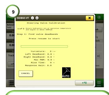
**9)** Move the wheel to the middle position and press either the engage button and or the black softkey engage button to start the calibration process. Follow the on-screen instructions, every step will require the engage button to be pressed to start. NOTE: The wheels will automatically move in this routine, ensure no-body is near the machine.
