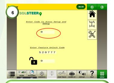
**6)** Access the setup and dealer lever diagnostics page. Enter the code 835 into the debug field.
