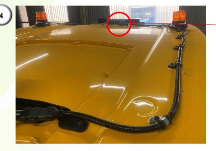
4) Plug the JCB/015 (9) into the 18 - way (male) at the rear of the roof. Secure the harness long the side of the roof.
