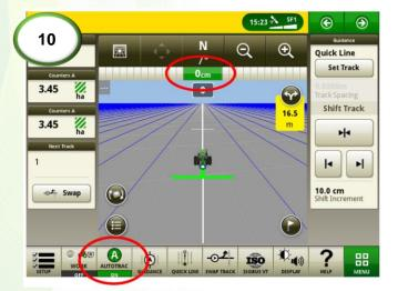
**10)** When calibration is complete, engage the steering and drive at about 4kph. Wait for the cross-track error to be holding a stable value around 0cm.
