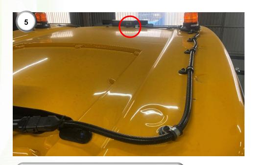
**5)** Fasten the cable along the roof and plug the opposing end into the machine (Rear of the cab - circled red).
