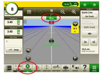
**8)** Engage the steering and drive at about 4kph. Wait for the cross-track error to be holding a stable value around 0cm.
