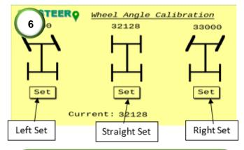
6) Calibrate the wheel angle sensor (WAS) limits. Ensure the current reading angle is not reading 0. Turn the steering wheel full lock left and press the left set button. Turn the wheel full lock right and press the right set button. Turn the wheel to dead straight and press the straight set button. Check the values above each set point to see if they've changed. Repeat the straight calibration
