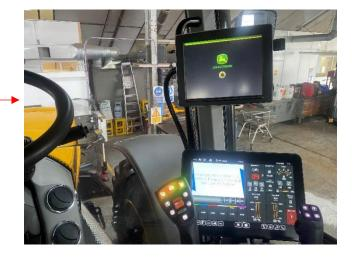
**3)** Plug the JCB/014 harness into the bottom of the 'A-Pilar' (circled green) and the opposing end into your mounted GreenStar display (as shown above)
