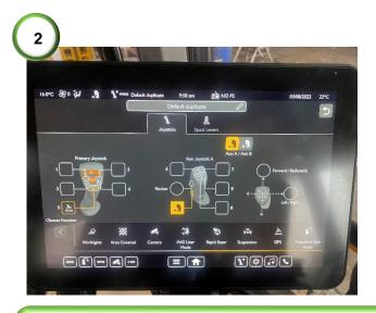
**2)** Assign the engage button to one of the buttons on the main control joystick.
