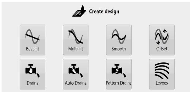
Enter all parameters to create design (refer to T3RRA Manual for detailed design information). NOTE: If you have a drain/field combination to design, always design the field first and the drain second.
