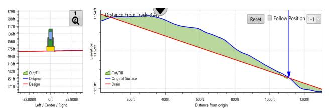
The right section of the screen shows design heights and original heights for the drain's full length. The blue arrow points to your current location and indicates the height of the blade. The red line in the diagram is the designed drain, the blue line shows the pre-implementation level of the ground and the green shading is area that will either be cut or filled. With this diagram you will be able to see cut depths along the length of the drain and estimate the number of passes required.
