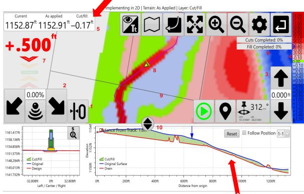
At the left side of the map screen there are a grouping of up/down chevrons that show the current blade height relative to the target design height. They show how far the blade needs to move, and in what direction, in order to be "on grade".
