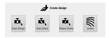
Enter all parameters to create design (refer to T3RRA Manual for detailed design information). NOTE: If you have a drain/field combination to design, always design the field first and the drain second.
