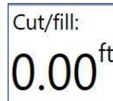
After placing implement's cutting edge on the ground, verify the selected SCV (1 and/or 3) is in Auto. Note: Manually adjusting blade height with SCV disables Automatic Control. Returning SCV to detent automates control.
